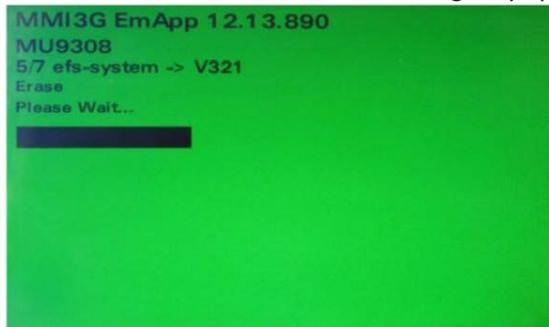
**Please Note:** The deletion and programming processes are performed several times, until all components of the MMI have been updated. Wait until the programming process is finished and the system automatically restarts. Your input is not necessary, the flash tool will begin deleting all the existing flash information in this step.
