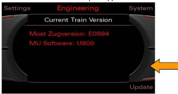
**Note:** You can quit the software download process at any time by simultaneously pressing and holding the Tone and Back buttons for more than five seconds.
