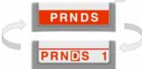
The warning displays signal to the driver to abort and retry the current operation (refer to description of overload protection or Software Shift Lock).
