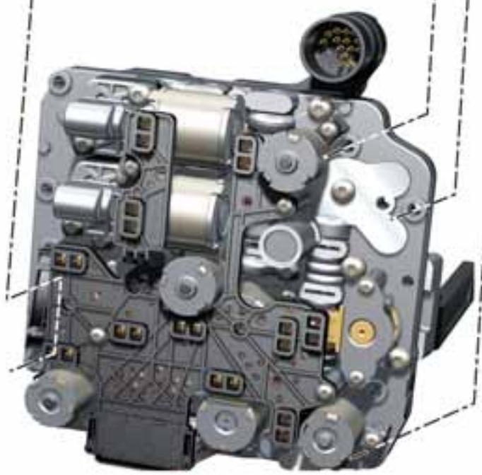
**Electro-hydraulic control unit with channel plate and PCB**
