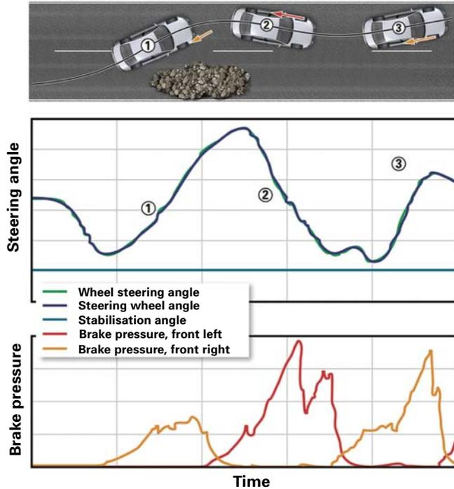
With the dynamic steering system, stabilising counter-steer is applied automatically, without the driver noticing anything. This significantly reduces the steering effort required on the part of the driver. The driver need only apply the steering angle that would be necessary in a similar, stable driving situation.
