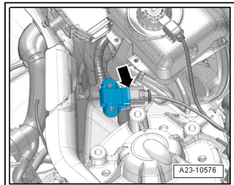
**Fitting location of pressure differential sender -G505-**
