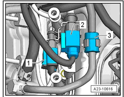
**Fitting location of fuel metering valve -N290-**
