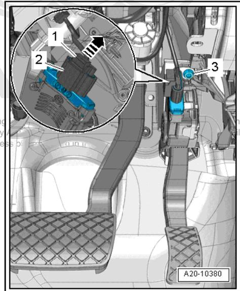
**Fitting location of brake light switch -F-**
