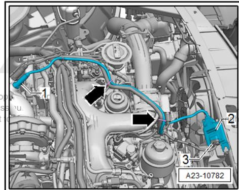
**Control unit for NOx sender 2 -J881- with NOx sender 2 -G687-
