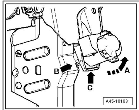
**Fitting location of brake servo pressure sensor -G294-**
