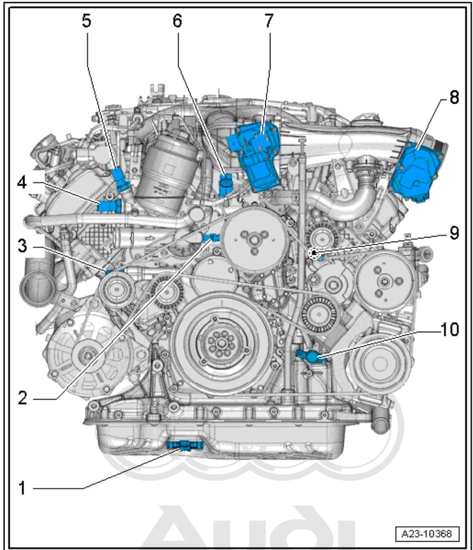
**9 - Temperature sender for engine temperature regulation -G694-**
