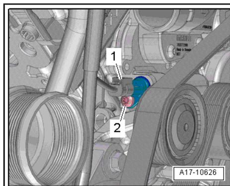
**Valve for oil pressure control -N428-**
