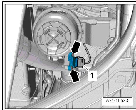
**Fitting location of temperature sender for engine temperature regulation -G694-**
