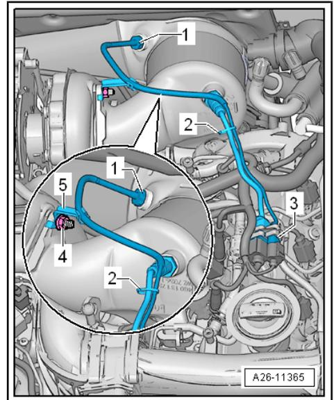
**Exhaust gas temperature sender 4 -G648- -arrow- (engine codes CMHA, CPNA only)**
