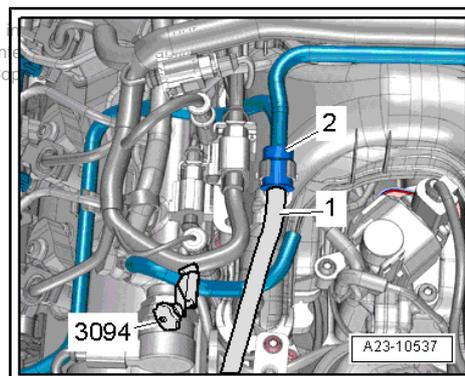
If specification is exceeded, this indicates that one or more injectors are defective. You must then check the return flow rate from each injector individually.
