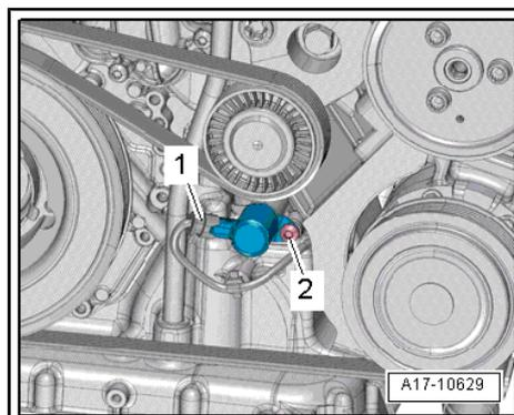
**Exhaust gas temperature sender 2 -G448- -1- (engine code CPNA only)**
