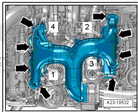
**4.2 Removing and installing intake manifold**
