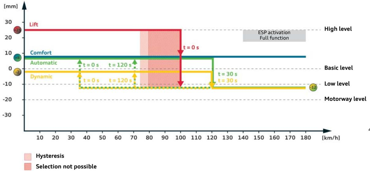
Control strategy - poor road running gear and suspension 1BY with trailer operation
