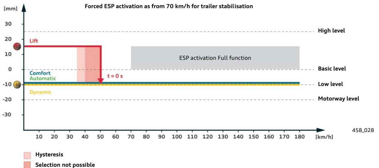
Control strategy - poor road running gear and suspension 1BY without trailer operation
