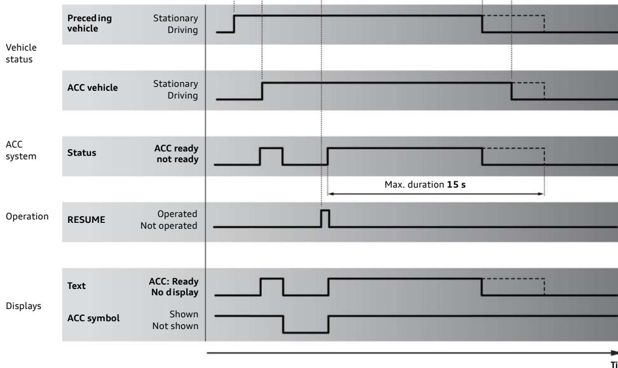
Example of the sequence of control operations in stop & go mode.
