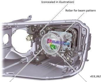
Dynamic cornering beam servo motor V318 (concealed in illustration)
