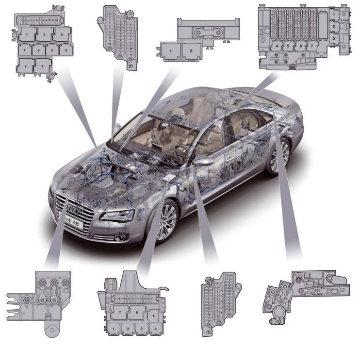
**Fuse box at forward end of longitudinal chassis member** This fuse box holds the fuses for the radiator fans.
