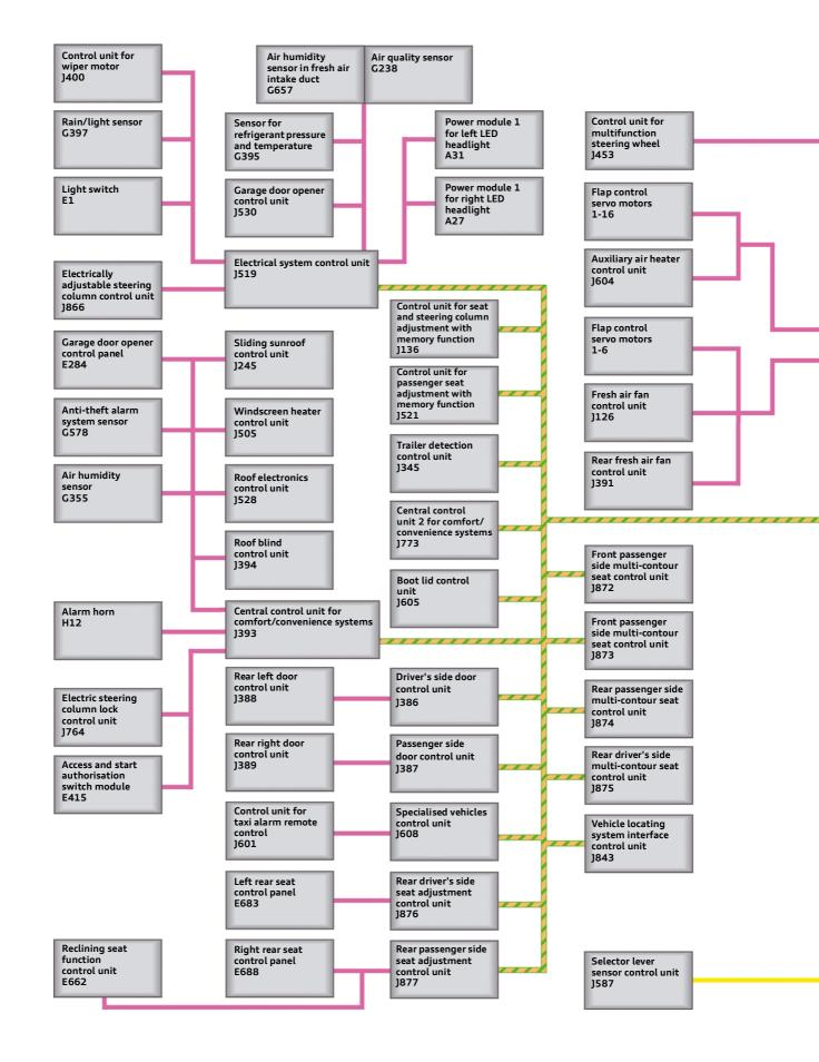
The diagram shows the network topology for a vehicle with an extensive level of optional equipment.
