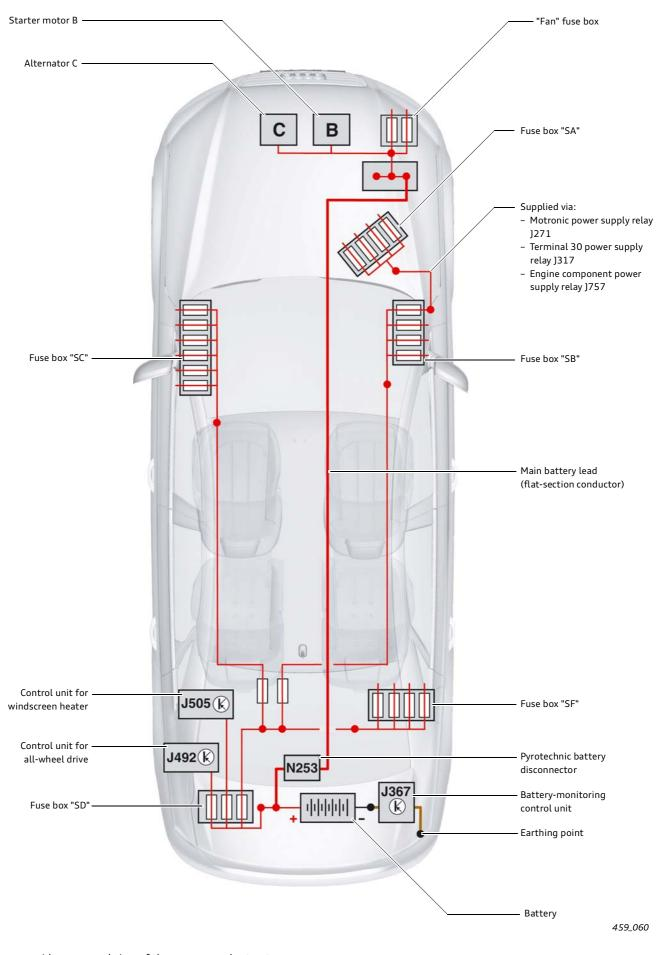
This diagram provides a general view of the power supply structure on the Audi A8 '10. It is a schematic diagram. For precise details of fuse assignment and cable routing, please
