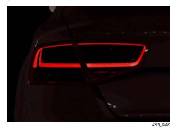
On the SAE version, the brake light is formed by a total of 72 LEDs.
