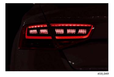
In addition, on the SAE version the top outer light strip section is switched off and the light strip dimmed to tail light level.
