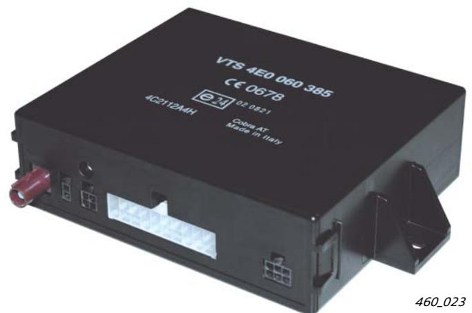
Vehicle tracking system control unit J895
