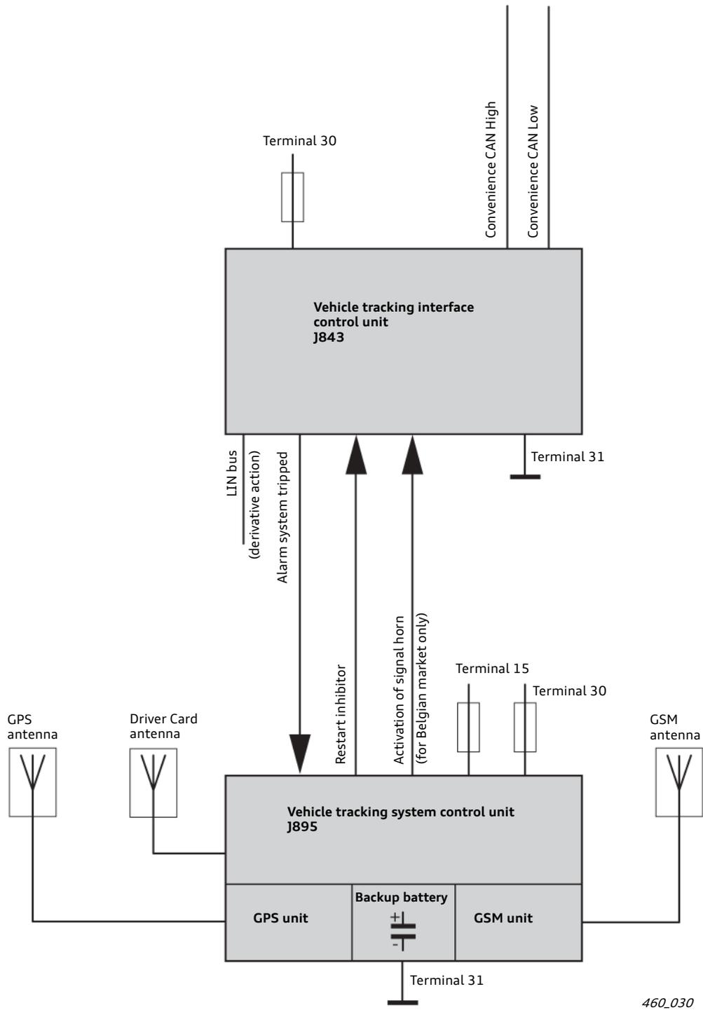
Audi tracking assist plus and connected antennas
