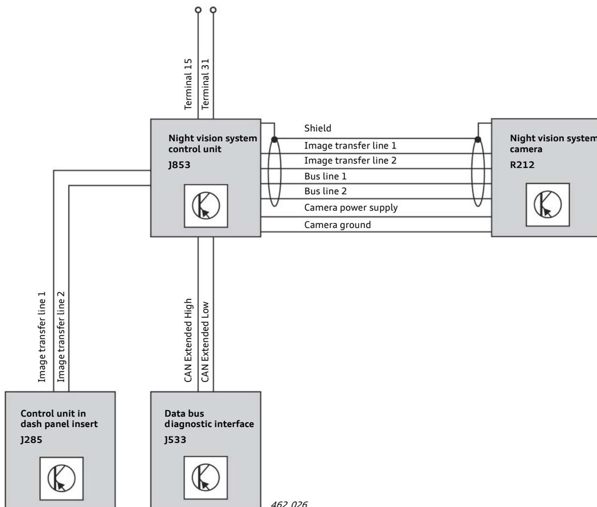
A sheathed and unshielded line with two twisted cores goes from the night vision system control unit J853 to the control unit with display in dash panel insert J285. An analogue video signal is transferred to the multi-functional display via this line.
