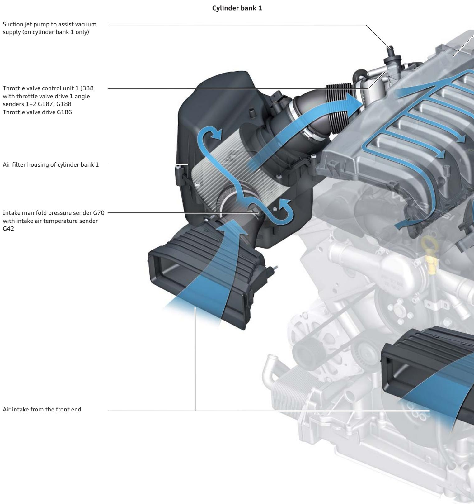
Compared to the intake system of the 6.0l W12 engine, the system on the 6.3l W12 FSI engine has undergone several major modifications. For example, the entire secondary air system is located at the back of the engine directly on the gearbox (see page 20).
