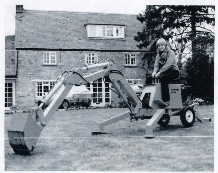
The Micron packs the quality, strength and experience from Fleming tractor mounted excavators into a compact versatile digger. Small enough to fit through 0.70m doorways yet with power to dig down a m effortlessly.
