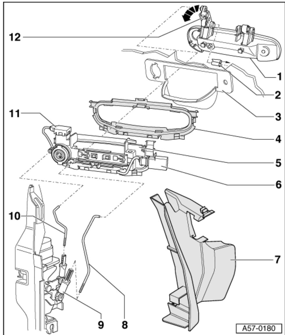
**10. Lock cylinder securing rod**
