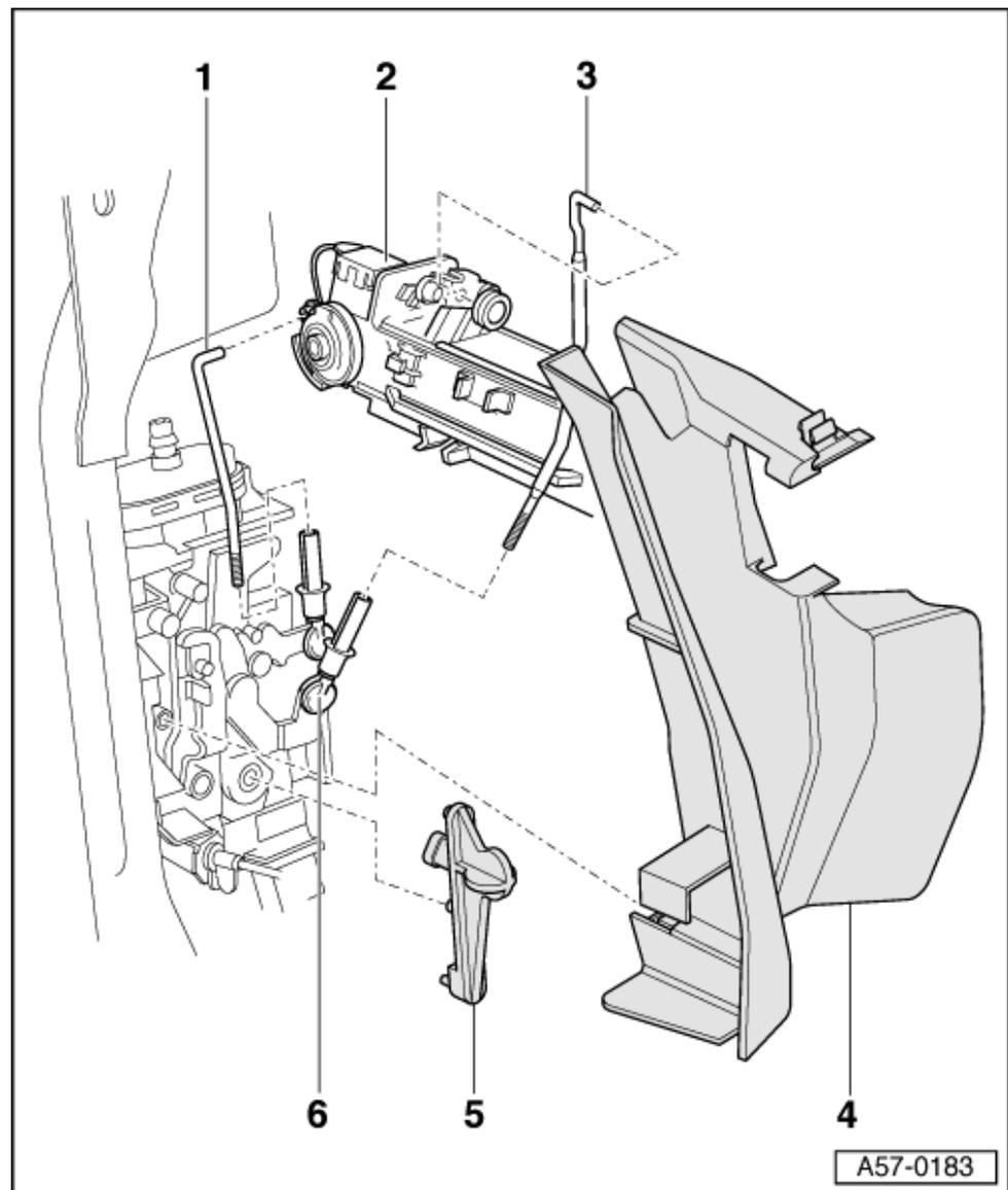
→ Fig.1 Removing and installing microswitch
