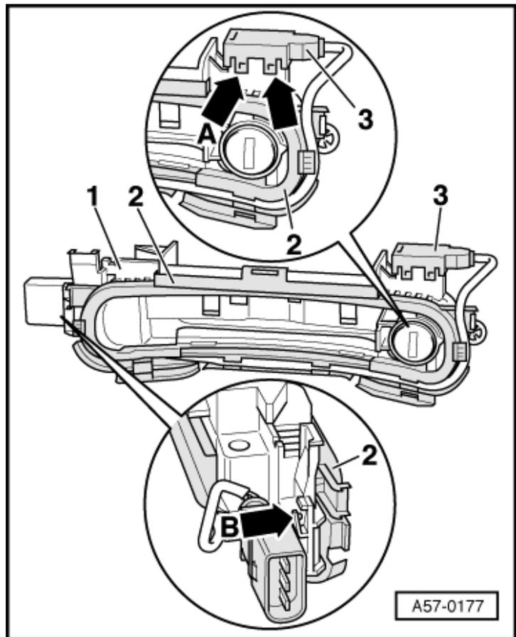
→ Fig.2 Removing and installing door handle seal
