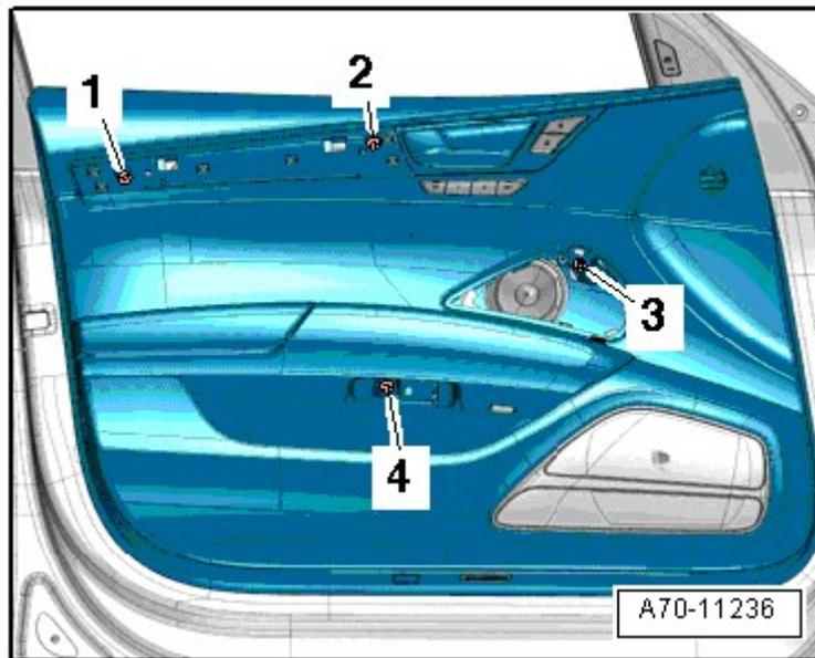
A two-piece clip is fitted at the bottom centre of the door trim. This clip must be released before unfastening the seven “normal” one-piece clips.
