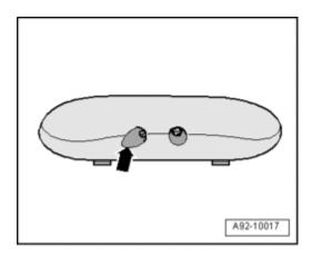
\* Oval opening - arrow - for single nozzle must point toward outside of vehicle.
