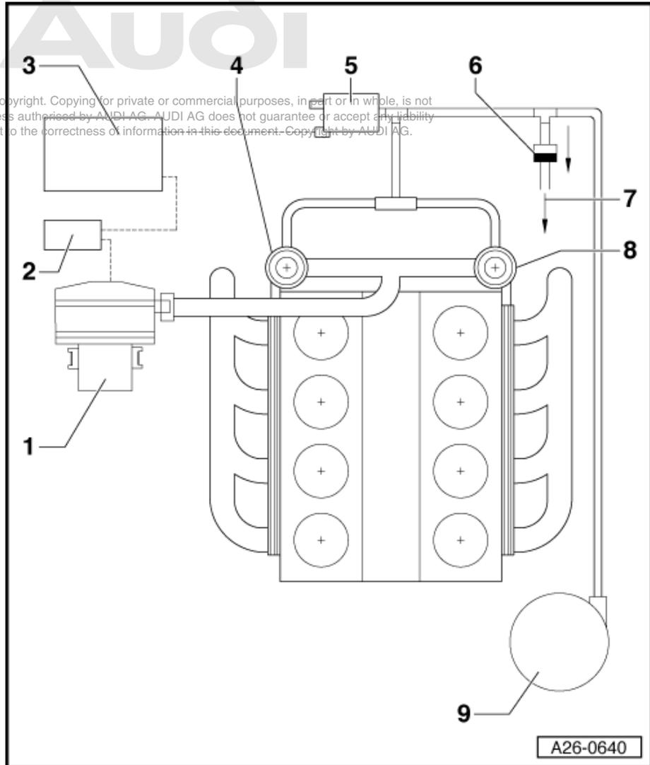
**Fitting location of secondary air inlet valve -N112-**
