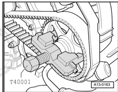
Installing (adjusting valve timing)
