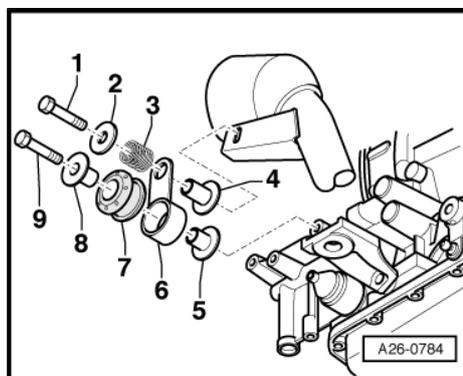
**Components of exhaust pipe mountings (right-side)**
