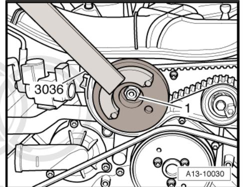
**Pulling off toothed belt sprocket for high-pressure pump**
