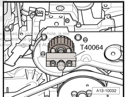
**Tightening union nut for high-pressure pipe at high-pressure pump**
