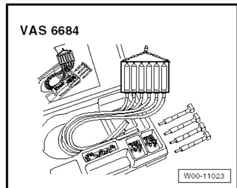
Checking return flow rate of all 6 injectors
