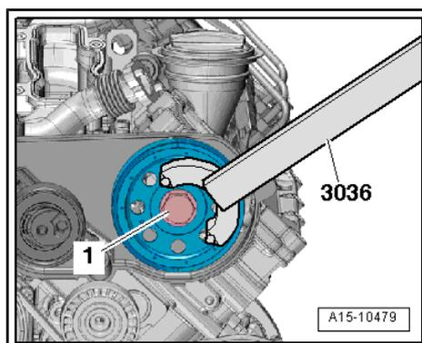
Turn crankshaft one complete revolution to check toothed belt tension. To do this:
