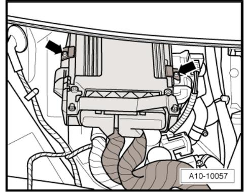
Remove retaining clip and engine control unit from electronics box (plenum chamber).
