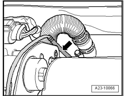
**Exhaust gas temperature sender 2 for cylinder bank 1 - G448-1-**
