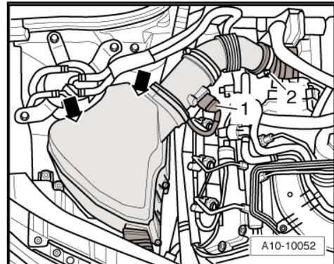
**1 - Connecting pipe for exhaust gas recirculation**
