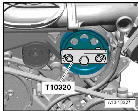
**1.25 Removing and installing toothed belt for high-pressure pump - vehicles up to 03.2006**
