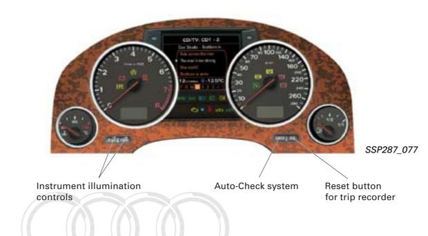
The dash panel insert in the Audi A8 '03 has been modified with respect to the predecessor model. Certain functions have been changed.
