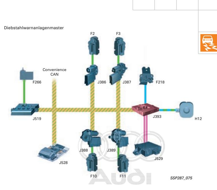
As anti-theft alarm master, the control units authorise 2, AUDI evaluates the corresponding vehicle<sup>ith respect to the corre</sup>F3<sup>ess of it</sup> monitoring information and actuates the antitheft output media as required.
