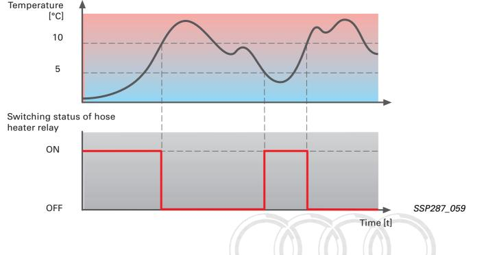
The windscreen washer system hose heater is actuated via a relay energised by the onboard power supply control unit 2 J520.
