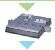
The onboard power supply control unit J519 actuates the following loads:
