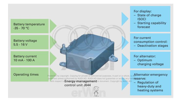
The battery current and battery temperature are measured in the control unit and the battery temperature converted to the battery by means of an algorithm. The battery voltage on the other hand is measured at the battery positive terminal.
