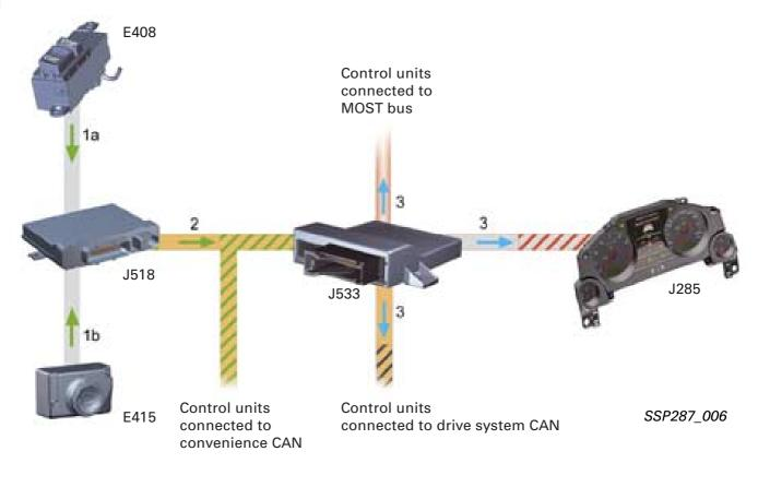
The data bus diagnostic interface J533 implements the exchange of data between the various data bus systems.
