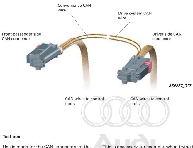
Use is made for the CAN connectors of the test box 1598/38.
