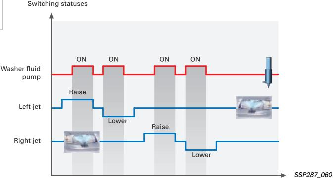
The onboard power supply control unit 2 J520 actuates one washer fluid pump and two pop-up washer jet motors. The washer fluid pump is actuated via the headlight washer system relay J39, which is energised by the onboard power supply control unit 2. The pop-up washer jet motors are switched directly by the control unit. As washing takes place during raising and lowering, the fluid jet is thoroughly distributed.
