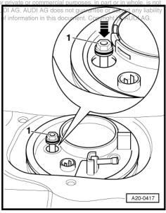
Pull fuel delivery unit upwards by approx. 40 mm while moving it slightly backwards and forwards.
