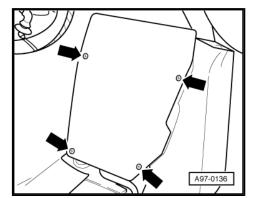
Pull auxiliary relay carrier out of guide rails -arrows 2- on both sides.
