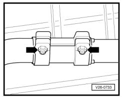
Remove bolts -arrows- and remove cover on underside of vehicle body (left-side).
