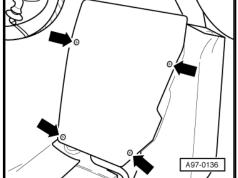
Pull auxiliary relay carrier out of guide rails -arrows 2- on both sides.
