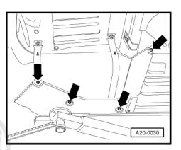
Remove bolts -arrows- and detach cover on underside of vehicle body (right-side).
