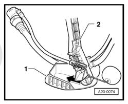
Look down the side of the opening into the fuel tank -arrowwhen inserting the sender.
