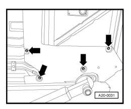
Detach 2-pin electrical connector -2- from bracket, release and unplug.
