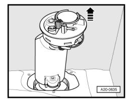
Pull fuel delivery unit out of fuel tank in position shown in illustration.
