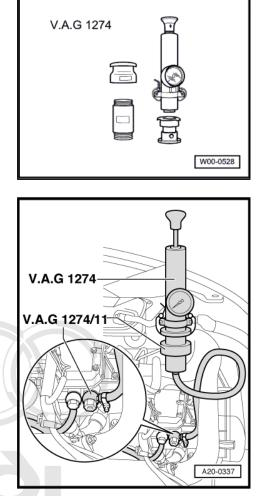
Using hose clamps -3094- , clamp off fuel hoses at the following points:
