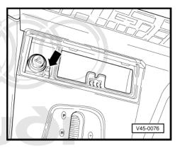
With ignition switched off, connect vehicle diagnostic, testing and information system -VAS 5051B<sup>Protected</sup> by copyright. Copying for private on permitted unless authorised by AUDI AG. AU with respect to the correctness of information
