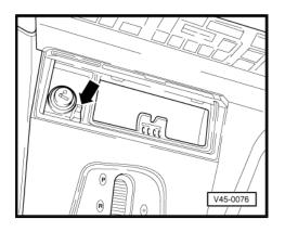
With ignition switched off, connect vehicle diagnostic, testing and information system -VAS 5051B- .
