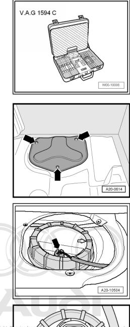
Release and unplug electrical connector for fuel gauge sender -arrow- at right flange.
