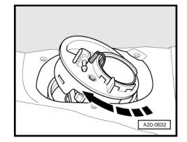
Turn fuel delivery unit approx. 45° further in clockwise direction while pulling upwards.
