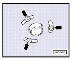
Release fasteners -1- and remove front noise insulation.
