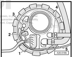
Unscrew union nut using union nut tool -T40068 A- .
