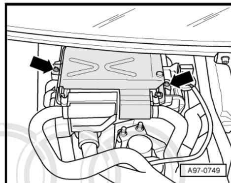
To help prevent unauthorised access to the connectors on the engine control units, the engine control unit -1- is bolted to a protective casing -4- by means of shear bolts -3- and a locking plate -2-.
