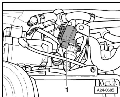
**Secondary air pump (beneath right-side longitudinal member)**
