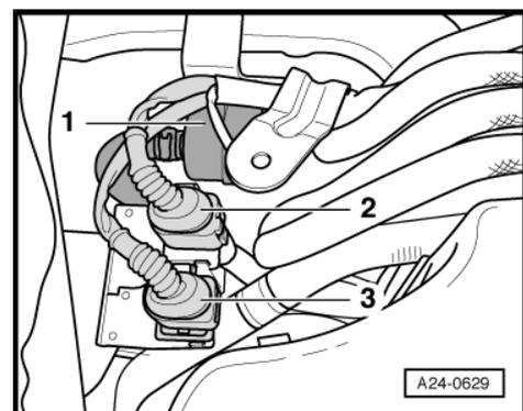
**Electronics box in plenum chamber**
