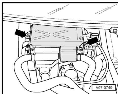
To help prevent unauthorised access to the connectors on the engine control units, the engine control unit -1- is bolted to a protective casing -4- by means of shear bolts -3- and a locking plate -2-.
