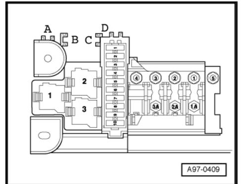
**4-position relay carrier in electronics box in plenum chamber**
