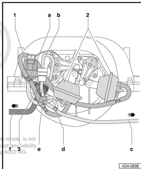
**Secondary air inlet valve -N112-**
