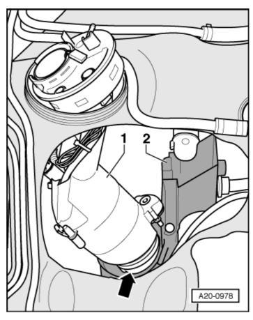
$-\to$  Now turn fuel delivery unit anti-clockwise 45°, which will lower the delivery unit into the fuel tank.
