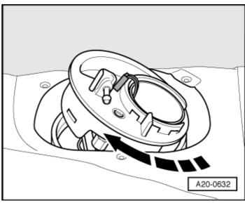
$- \rightarrow$  Turn fuel delivery unit clockwise  $45^{\circ}$  more while pulling upwards.
