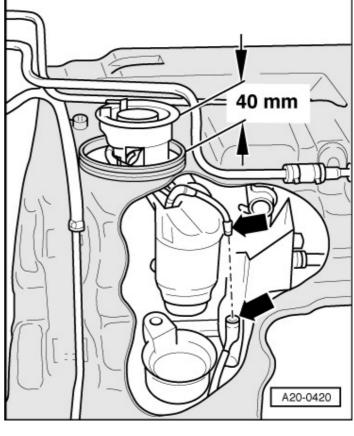
After checking the installation, lift out fuel delivery unit approx. 40 mm.
