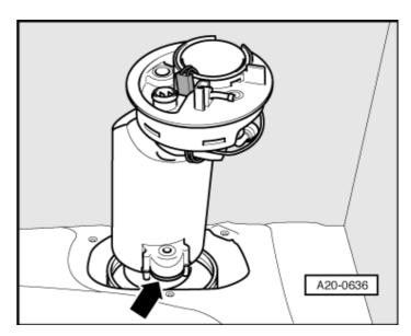
→ Place fuel delivery unit in fuel tank and turn clockwise approx. 90°.
