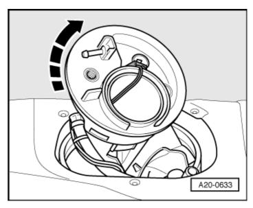
$- \to \text{Now turn fuel delivery unit anti-clockwise} 45^{\circ}$  while pulling upwards...
