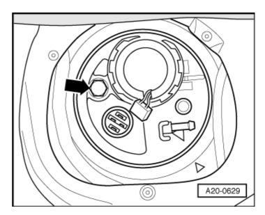
$- \rightarrow$  Fit locking ring and tighten to 70 Nm using special tool 3342.
