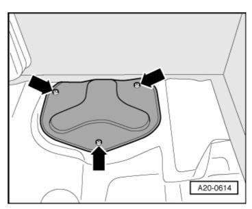
— Using special tool 2012 A, release flange for fuel gauge sender by turning it clockwise, detach flange and take out the spring below it.
