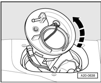
$- \to \text{Turn}$  the fuel delivery unit anti-clockwise 45° further to its fitting position.
