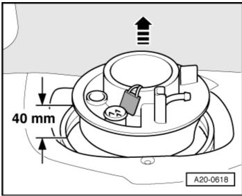
$- \rightarrow \mbox{Remove}$  flange seal from edge of opening.
