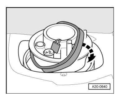
$- \rightarrow$  Fit new O-ring -1- on securing bolt -2-.
