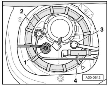
– → Unscrew and remove union nut with special tool 3342.
