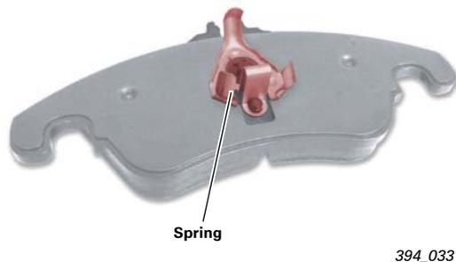
The brake pad wear indicator sensor is located in the front left wheel brake pad. The signal from this sensor is read in by the onboard power supply control unit J519.
