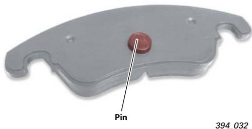
The brake lining on the piston side is held in place in the brake piston by a stainless steel spring.
