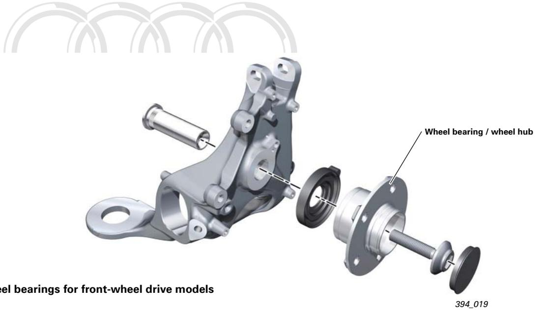
Wheel bearings for front-wheel drive models
