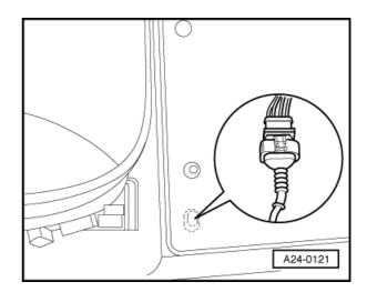
$\rightarrow$  The four-way connector for lambda probe 2 (G131) bank 2 is under the mat on the driver's side.
