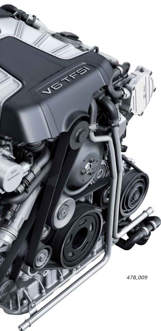
Adapted belt drive (without power steering pump)
