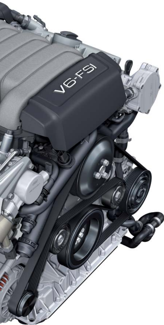
Adapted belt drive (without power steering pump)
