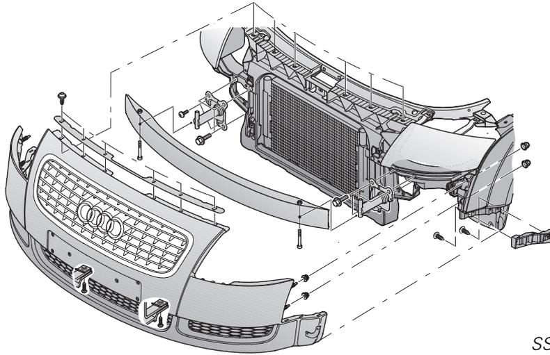
The front bumper comprises two parts: the cover panel and a decorative grille. The bumper carrier is made of aluminium and bolted to the side members by impact absorbing elements.
