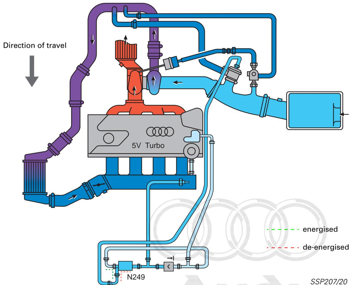
The turbocharging system comprises the following components:
