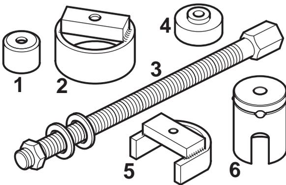
**Wheel bearing puller for quattro rear axle**
