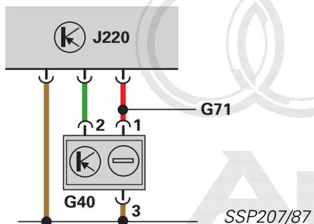
The Hall sender G40 is connected to the sensor earth terminal of the engine control unit.
