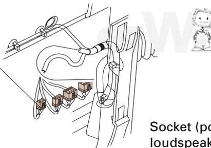
Socket (power windows, loudspeaker, radio, central locking, anti-theft alarm)
