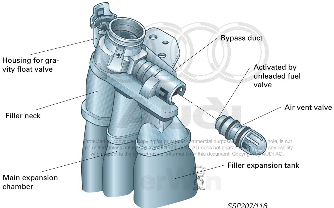
When refuelling the vehicle, the unleaded fuel valve activates the air vent valve. The valve seals the main expansion chamber so that no fuel vapour can escape from this tank when the vehicle is being refuelled. The filler expansion chamber is vented by the filler neck.
