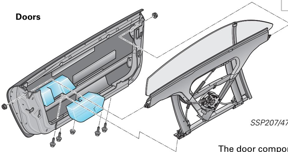
The doors of the Audi TT Coupé are frameless and of two-piece construction.
