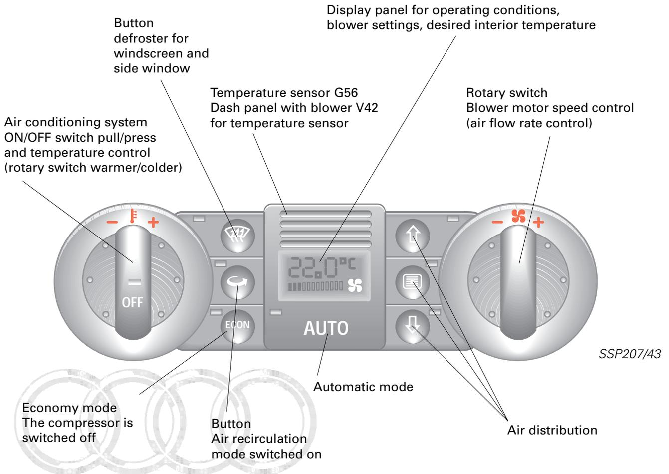
The fully automatic air conditioning system operates according to Audi's tried and tested principle. The sensors and actuators provide automatic temperature and air flow rate control.
