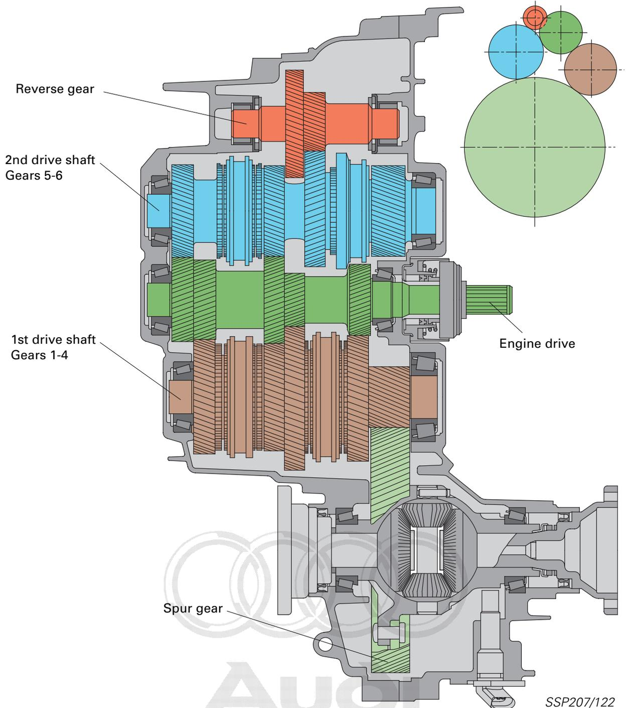
**!** The spur gear is riveted to the differential. For more detailed information on the manual gear-boxes, see SSP 205. If repair work is necessary, the spur gear must be bolts.
