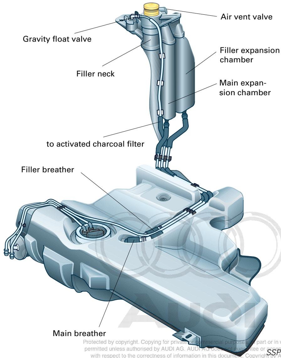
When refuelling the fuel tank, the gas mixture is conveyed via the filler breather directly into the filler expansion chamber and from here via the filler neck into the atmosphere.
