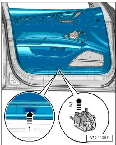
A two-piece clip is fitted at the bottom centre of the door trim. This clip must be released before unfastening the seven "normal" onepiece clips.
