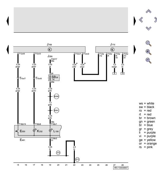
Lane change assist control unit, lane change assist control unit 2, button for lane change assist, lane change assist warning lamp
