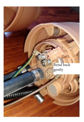
Bend the two retaining clips located on opposite sides of the fuel pump out of the way and the fuel pump can be withdrawn from the lower part of the housing by pulling on the hose attached to the pump spiggot. I found it to be a very tight fit so go easy, as you wouldn't want to break anything. Did i mention that already? Install the new pump, connect the wires, put the hose clamps on and then reassemble the housing.
