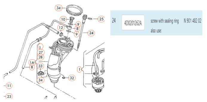
The 12" long bolt (number 24 in the diagram above) required a lot of torque to unfasten so I put a piece of galvanised iron pipe over the socket wrench handle so that I had more leverage and control over the motion of the wrench. I have read several stories of woe saying that the captive nut where the long bolt fastens to at the bottom of the fuel tank broke in its plastic housing and the bolt subsequently being unable to be released.
