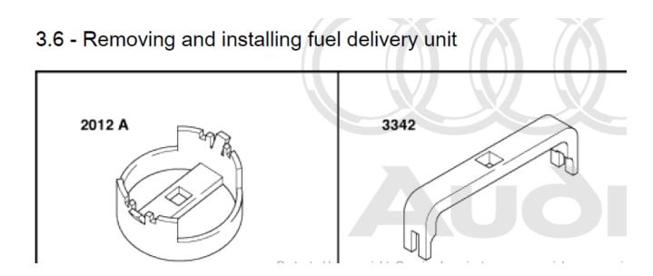
10mm bolts and nuts to suit mounted and spaced on a piece of slotted right angle metal of some description served as a DIY version of Audi special tool 2012A A clockwise twist saw the cap released
