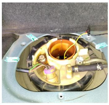
I made some marks on the pump housing and on some tape stuck to the boot floor so that I could be sure that the pump housing was oriented correctly upon reinstallation. I asm not sure it was necessary, as the housing can really only be in a certain position when seated correctly. It was reassuring though.
