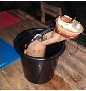
Lift the housing straight up whilst turning gently left and right. This releases the housing from the plate at the bottom of the tank. Then turn the housing anti-clockwise whilst lifting.
