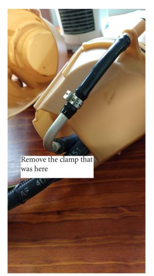
After you remove a clamp you can remove the hose hose coming from the fuel pump from the boomerang and then the upper housing can be slid away from the lower part thus allowing access to the fuel pump.
