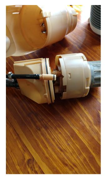
You can't separate the two halves of the fuel pump enclosure until you remove a clamp from the metal boomerang shaped fuel connector that attaches to the hose coming from the fuel pump.
