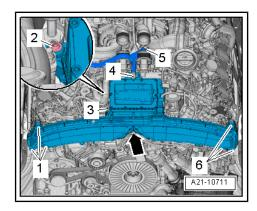
Remove coolant pipe (top left) ⇒ Engine, mechanics; Rep. gr.
