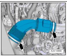
Remove bolts -arrows- and push wiring guide -1- slightly to right side.
