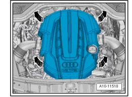
Vehicles with engine code CEUA: Release hose clips -arrows- and remove air pipe.
