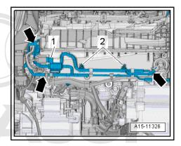
Unplug electrical connector -arrow- for fuel pressure sender -G2'47- . permitted unless author with respect to the
