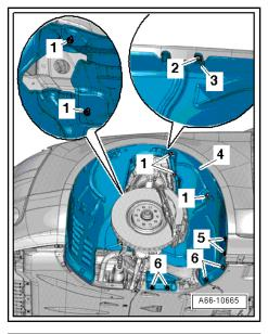
Remove bolts -arrows- and detach heat shield for drive shaft (right-side).
