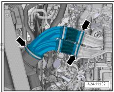
Vehicles with engine code CGTA: Release hose clips -arrows- and remove air pipe (right-side).
