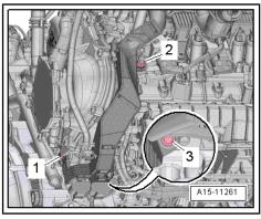
Unscrew centre hex stud -arrow- and remove guard plate -1-.
