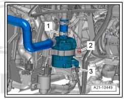
Fitting location of coolant valve for gearbox in N488 vate or commercial purpose permitted unless authorised by AUDI AG. AUDI AG does not guar
