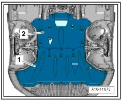
Remove front underbody cover -2- (left and right)  $\Rightarrow$  General body repairs, exterior; Rep. gr. 66 .
