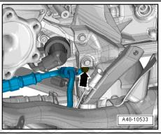
Remove bolts for gearbox mounting -arrows- on both sides.
