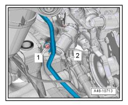
Remove electrical connector -2- for Servotronic solenoid valve -N119- from bracket and unplug connector:
