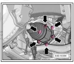
Remove nuts -1, 2- and bolt -3-, move wiring guide clear and push to one side.
