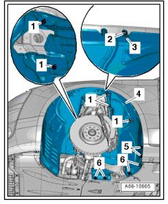
If fitted, release clamp -2- and detach exhaust silencer -1- for auxiliary heater.
