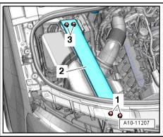
Vehicles with engine code CEUA: Release hose clips -arrows- and remove air pipe.
