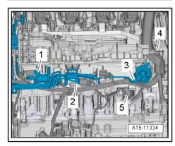
Unplug electrical connector -2 for intake manifold flap poten to tiometere2 te6512 ectness of information in this document. Copyright by AUDI AG.
