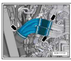
Vehicles with engine code CGTA: Release hose clips -arrows- and remove air pipe (right-side).
