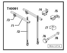
Engine support bracket (supplementary set) -T40093- with -T40093/7- and -T40093/8-
