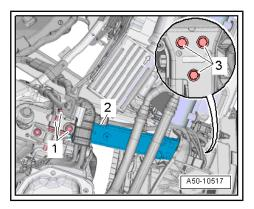
Remove bolt -4- for battery positive wire -3- and bolt -2- for earth wire -1- and move electrical wiring clear.
