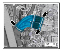
Vehicles with engine code CGTA: Release hose clips -arrows- and remove relevant air pipe.
