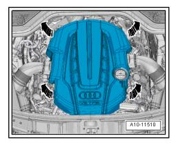
Vehicles with engine code CEUA: Release hose clips -arrows- and remove air pipe.
