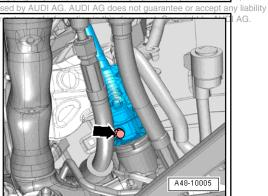
Detach intermediate steering shaft from steering rack and pect to the c slide splines together ⇒ Rep. gr. 48.
