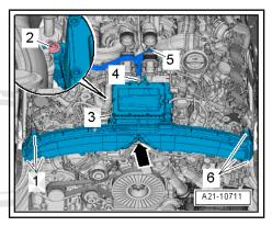
Detach charge pressure control solenoid valve -N75--item 2- from bracket -1- and push it clear to one side.
