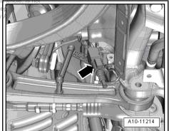
Remove bolt -1- for anti-roll bar on both sides.
