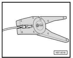
Slide a "yellow" crimp connector -2- from wiring harness repair set -VAS 1978- onto free ends of vehicle wiring harness -1and Y wire -3- for coolbox.
