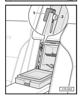
Install trim frame for coolbox, pressing it on carefully -arrows-.
