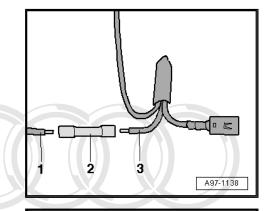
Use crimping pliers -VAS 1978/1- to crimp the crimp connector with the "yellow" crimp recesses on both sides.
