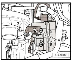
Install new intake manifold flap motor - V157- in reverse order of removal and clip coupling rod on.
