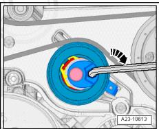
Tension tensioning roller slightly from "3 o'clock" position -arrow- until lug -1- and notch -2- are exactly in line.
