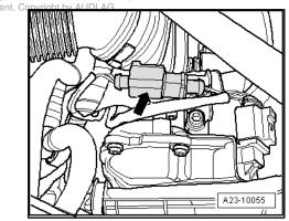
Disconnect connecting wire - VAS 6395/4-2- -item 3- from intake manifold flap motor - V157-.
