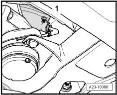
Exhaust gas temperature sender 2 for cylinder bank 1 - G448-
