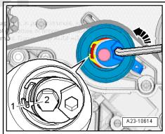
Tension tensioning roller slightly from "3 o'clock" position
