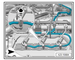
Disconnect fuel return hoses from injectors on cylinder bank 2; to do so, press down both tabs and at the same time pull centre piece up to release connection -arrow-.
