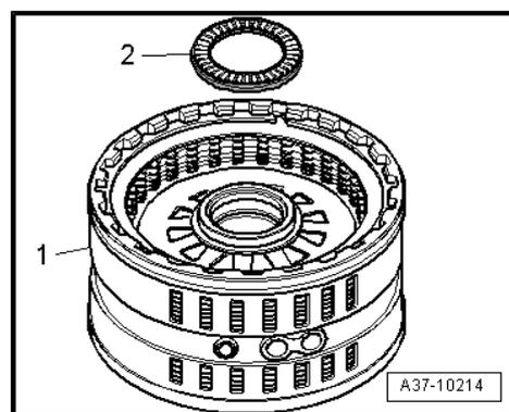
– Detach circlip -1- and remove clutch pack -2- from cylinder „E“.
