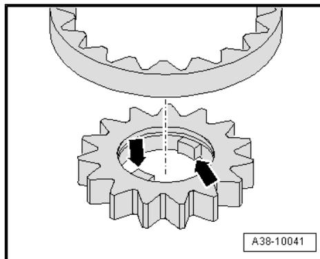
A - Installation incorrect: torque converter not inserted properly when installing gearbox or engine. Check installation depth ⇒ [page 13](#) .
