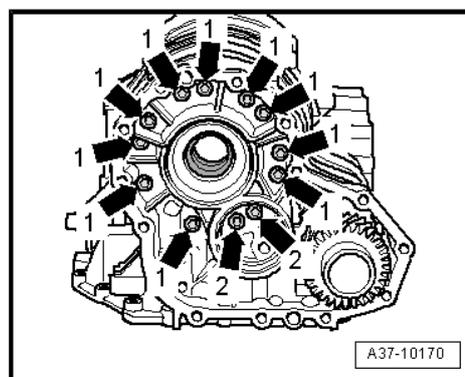
**Tightening sequence for gearbox with countersunk head bolts**
