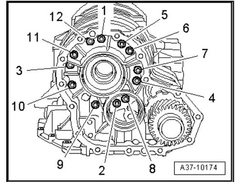
**Tightening sequence for gearbox with oval-head bolts and countersunk head bolts**
