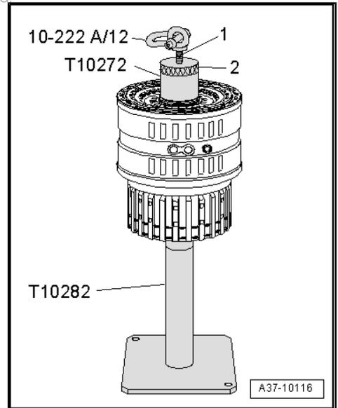
– Detach clutch „C“ -item 2- with sun shaft from cylinder „D/E“ -item 1-.
