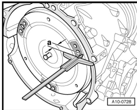
B - Installation incomplete: torque converter centring sleeve -arrow- not inserted in crankshaft ⇒ Engine, mechanics; Rep. gr. 13
