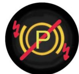
System fault; vehicle should no longer be driven for safety reasons.
