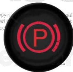
Fault detected by control unit restricting operation.
