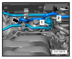
Detach vacuum hose -arrow- going to intake manifold connection.
