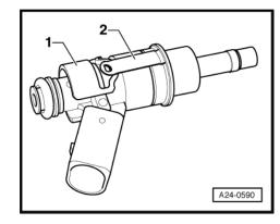
Fit assembly cone -T10133/5- with new combustion chamber ring seal -1- onto injector -2-.
