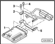
The threads of the two shear bolts -4- which are not screwed into the engine control unit are secured with locking fluid. To unscrew these two bolts, the threads must therefore be heated with the hot air blower.
