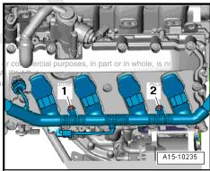
Pull ignition coils out of spark plug apertures using puller -T40039- .
