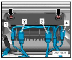
Unscrew Lambda probe -G39- -item 2- and Lambda probe after catalytic converter -G130- -item 1- using a tool from the Lambda probe open ring spanner set -3337- .
