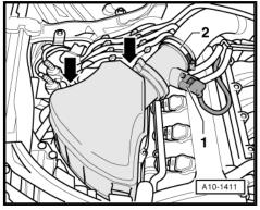
Unscrew bolts -arrows- from air cleaner housing and detach top section of air cleaner housing.
