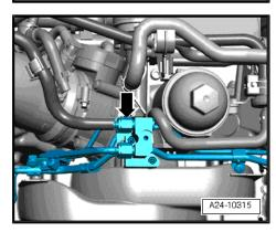
Disconnecting fuel supply pipe -arrow- from connecting piece (engines with plastic intake manifolds)
