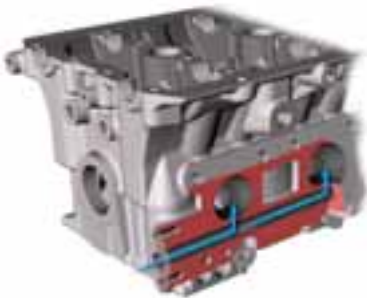
Additional air flows through a port in the cylinder head to each exhaust port in order to burn the rich fuel-air mixture downstream of the exhaust valves after cold starting (catalytic converter start).
