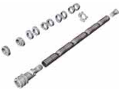
To reduce the weight of rotating parts, the camshafts are manufactured from a hollow tube and mount-on cams.
