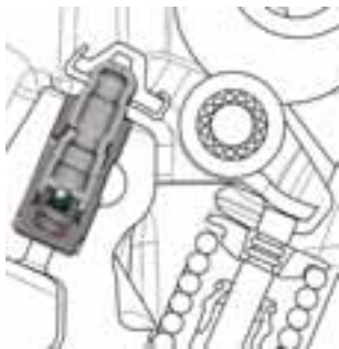
Hydraulic valve clearance compensation elements are supplied with hydraulic oil through transverse bores in the cylinder head and provide backlash free valve actuation.
