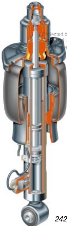
quattro drive Coaxial arrangement of air springs/PDC damper
