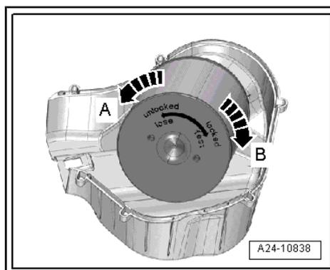
Continue installation in reverse sequence. Note tightening torque ⇒ [page 112](#) .
