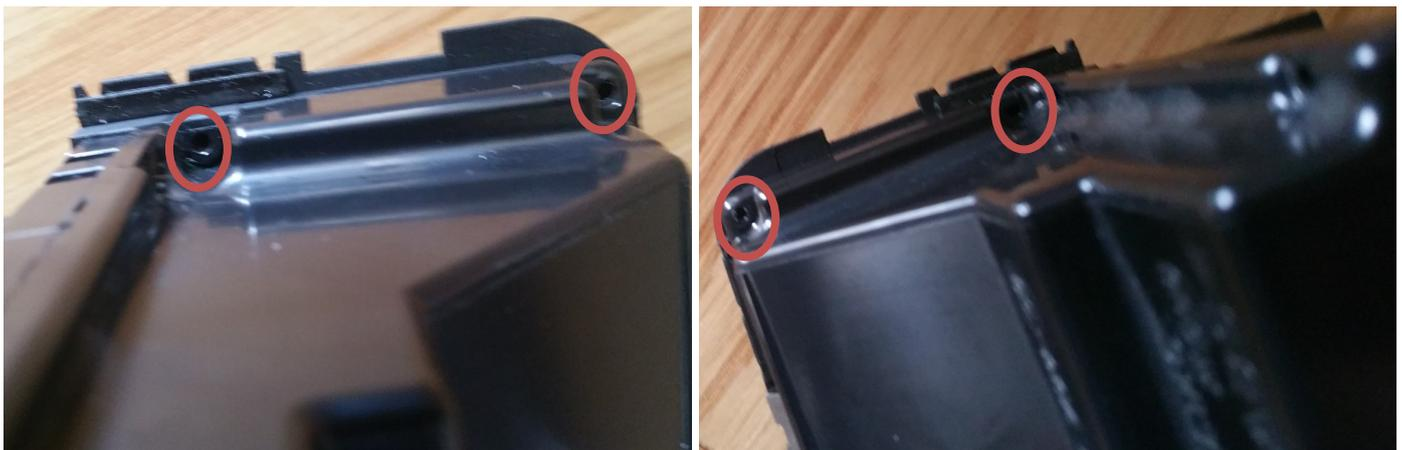
The front panel can now be taken from the case by lifting the four tabs, two on the top and two on the bottom.
