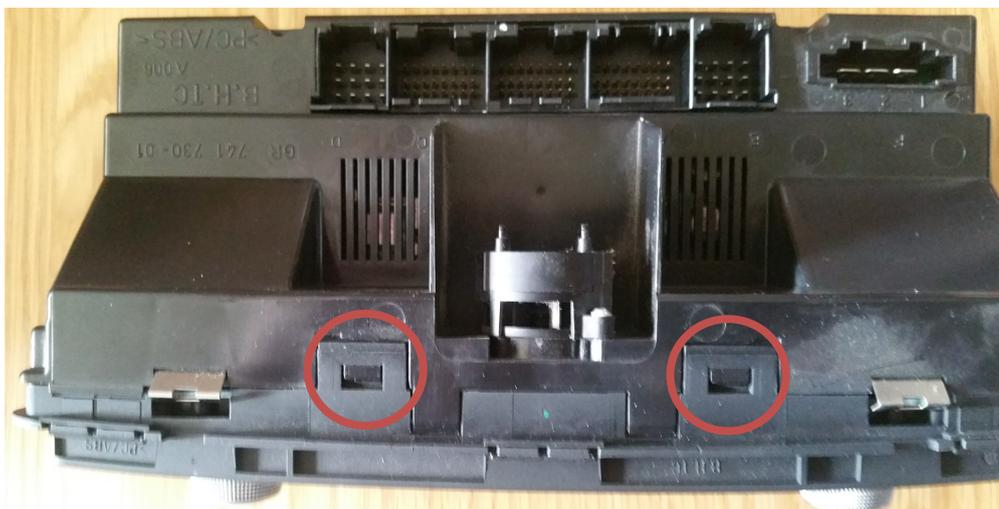
The remaining six T6 screws hold the two part case together.
