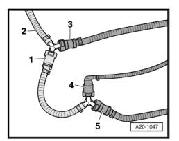
Working through left fuel tank opening, press release tabs -arrows- and detach fuel supply line -2-.
