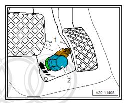
Disengage cap -2- of kickdown switch -1-; to do so turn cap anti-clockwise -arrow A-. Pull cap out as far as stop -arrow B-.
