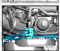
Disconnect fuel supply line -arrow- at connecting pieces authorised to be corrected to the corr
