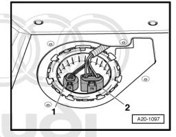
Unscrew locking ring using wrench - T10202- . \_
