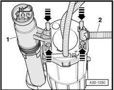
Working through left fuel tank opening, fit balance pipe -1- and supply line -2- going to suction-jet pump (right-side) and supply line -3- going to fuel delivery unit (left-side) so that they engage audibly.
