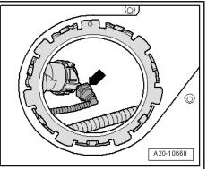
Working through left fuel tank opening, press release tabs and disconnect supply lines -2- and -3- for suction-jet pumps from Y-connector.
