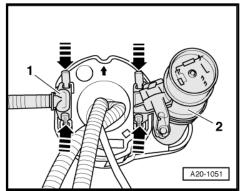
Working through right fuel tank opening, fit supply lines -1- and -2- for suction-jet pumps onto Y-connector so that they engage audibly.
