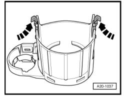
Fit fuel supply line -1- and fuel gauge sender 4 - G393--item 2- so that they engage audibly on fuel delivery unit (rightside).
