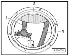
Fit fuel supply line -2- onto fuel delivery unit (left-side) so that it engages audibly.
