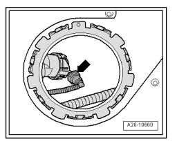
Working through left fuel tank opening, press release tabs and disconnect supply lines -2- and -3- for suction-jet pumps from Y-connector.
