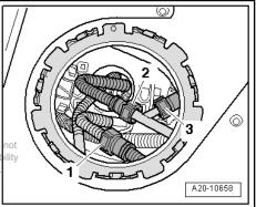
Working through right fuel tank opening, fit fuel supply line -2- so that it engages audibly.
