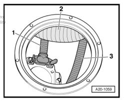
8 Fuel delivery unit with fuel pump and fuel gauge senders - USA vehicles with MPI engine
