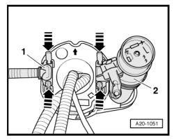
Fit fuel supply line -1- and fuel gauge sender 4 - G393--item 2- so that they engage audibly on fuel delivery unit (rightside).  Working through right fuel tank opening, fit supply line -1- going to suction-jet pump (left-side) and supply line -2- going to fuel delivery unit (right-side) so that they engage audibly.
