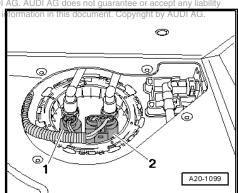
Connect hand-held multimeter between contacts -2- and -3of connector -A- to measure resistance.
