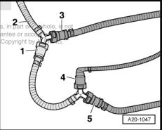
Working through right fuel tank opening, press release tabs -arrows- and detach fuel supply line -1- and fuel gauge sender 4 - G393- -item 2-. Move fuel gauge sender 4 - G393- to right side.
