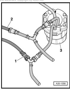
Unclip fuel filler pipe -arrow- at front of fuel delivery unit (rightside).
