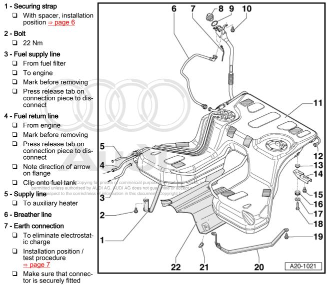
$\hfill \begin{tabular}{ll} \label{eq:alpha} \begin{tabular}{ll} After installation, use an ohmmeter to check the electrical connection between the fuel filler neck and a bare metal part on the body. Specification: approx. 0 <math display="inline">\Omega$
