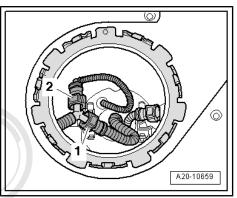
Working through right fuel tank opening, press release tabs -arrows- and detach fuel supply line -1-.
