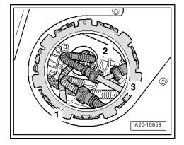
Working through right fuel tank opening, press release tabs and disconnect supply line -1- going to suction-jet pump (leftside) and supply line -2- going to fuel delivery unit (right-side).
