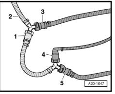
Connect electrical connectors -1 ... 3- on underside of flange (left-side).
