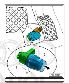
Lock cap -2- of kickdown switch -1- in place by turning cap 15° in clockwise direction -arrow- as far as stop.
