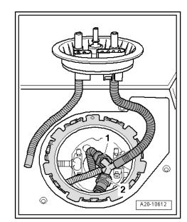
Working through right fuel tank opening, press release tabs and disconnect supply lines -1- and -2- for suction-jet pumps from Y-connector.
