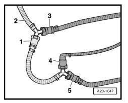
Working through left fuel tank opening, press release tabs -arrows- and detach fuel supply line -2-.
