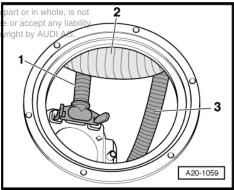
10 Fuel delivery unit with fuel pump and fuel gauge senders - USA vehicles with FSI engine
