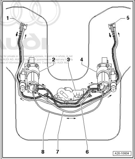
which the fuel pumps are fitted, as well as the fuel pumps themselves. The baffle housing is a container permanently filled with fuel, so that the fuel pumps are surrounded with fuel regardless of the fuel level in the tank.
