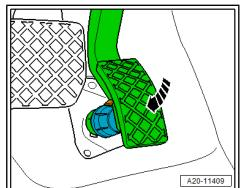
Press accelerator pedal down as far as stop -arrow- and release again.
