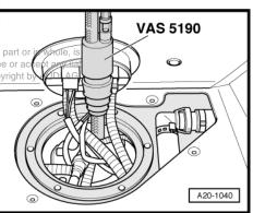
1.3 Removing and installing fuel tank with attached components
