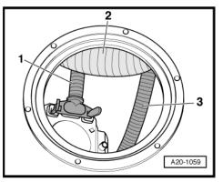
Fit fuel supply line -1- onto fuel delivery unit (right-side) so that the locking hooks engage audibly.
