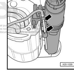
Connect electrical connectors -1 ... 4- at underside of flange.
