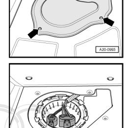
Connect hand-held multimeter - V.A.G 1526 E- between contacts -2- and -3- of connector -A- to measure resistance.
