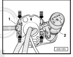
Fit fuel lines -2- through left opening on fuel tank so that they engage audibly.
