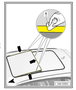
Use a sponge -1- to lubricate glass panel seal at front -arrow- with Krytox lubricating paste - G 052 141 A2-. Make sure that no coarse residue remains visible after applying lubricant.
