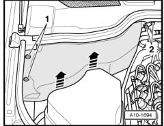
Remove securing bolts -arrows- and detach air cleaner (top section).
