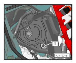
Remove securing bolts -arrows- from air cleaner (top section) and detach it.
