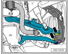
Check bonded rubber bushes -arrows- of track control links and guide links for play.
