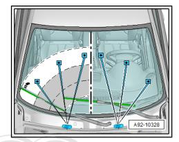
If water jet does not contact headlight: Renew relevant washer jets ⇒ Rep. gr. 92; Headlight washer system; Removing and installing washer jets.
