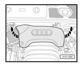
Carefully pull engine cover panel (front) off retaining pins one after another -arrows-.
