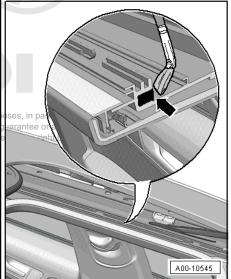
Apply lubricating paste - G 060 751 A2- to inside of guide rail -arrow- using paintbrush.
