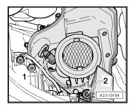
If no dirt was found: Pour a small amount of water into plenum chamber above engine cover panel (right-side) -arrow- and check that water drains quickly and fully.
