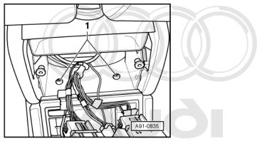
Remove rear air vent and screw out bolts -1-.
