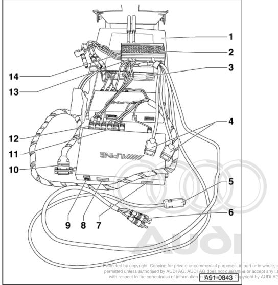
10 AUX2 cable to "AUX INPUT2" input at rear information display and operating unit control units -J648 and -J649
