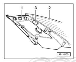
Two further aerial amplifiers are bolted on at top of right and left D-pillar.
