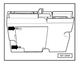
Back-up battery is only to be disconnected from control unit if it is to be replaced.
