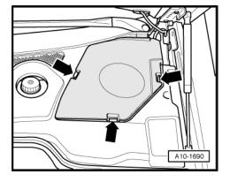
Vehicles with auxiliary heater: remove bolts -arrows- securing exhaust pipe for auxiliary/additional heater to noise insulation.
