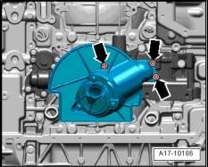
Unscrew bolts -arrows- and remove oil pipe together with housing for oil cooler bypass valve.
