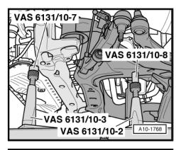
Tighten bolts for gearbox mountings -arrows- on both sides ⇒ Rep. gr. 37.
