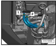
Disconnect coolant hoses -1- and -2- from auxiliary radiator (right-side) and drain off remaining coolant.
