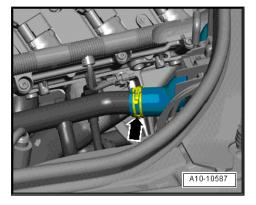
Remove bolt -arrow- on mounting for torque reaction support.
