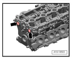
Use impact extractor attachment -T40116- to pull out locating pins -T10133/3-.
