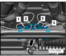
Take electrical connectors -1- and -2- for Lambda probes out of bracket and unplug connectors.
