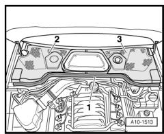
Unbolt bracket (left-side) for refrigerant line from suspension turret -arrow-.
