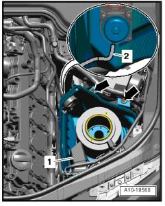
Extract hydraulic fluid for power steering from reservoir using used oil collection and extraction unit - V.A.G 1782- .
