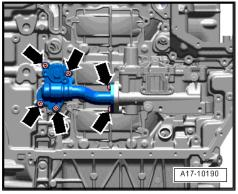
Remove bolts -arrows- and support oil pump by hand.
