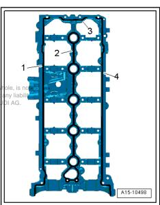
Insert locating pins -T40116- in retaining frame and in cylinder
