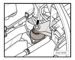
Unscrew bolts -arrows- and remove mounting for torque reaction support.
