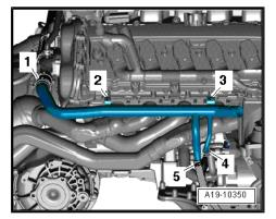
Unscrew bolt -arrow- at bracket for exhaust pipes (right-side).
