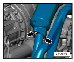
Unscrew nuts in the sequence -9 ... 1- and remove front right exhaust manifold with catalytic converter.
