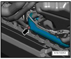
Disconnect coolant hoses -1 ... 3- and drain off coolant.
