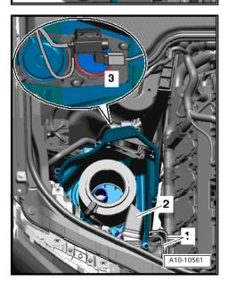
Detach coolant hose (right-side) -arrow- at engine.
