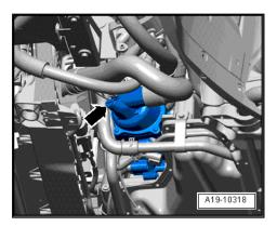
Install drain plug -arrow- with new seal on front coolant pipe.
