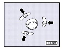
Open quick-release fasteners -1- and remove noise insulation (front).
