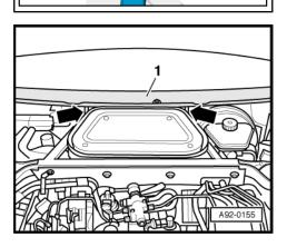
Unbolt cross piece for suspension strut -arrow-.
