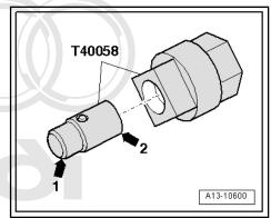
Using adapter - T40058- turn the crankshaft in the normal diudiag rection of rotation -arrow- to "TDC"
