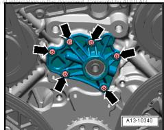
Install bearing cover (front) -arrow- for balance shaft.
