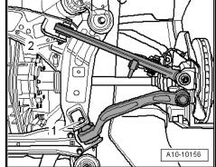
Pivot guide link -1- and track control link -2- outwards.
