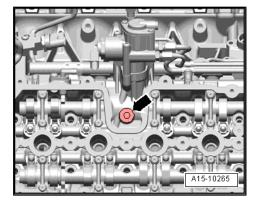
Make sure that guide rail of chain tensioner for camshaft timing chain is locked with locking pin - T40071- .
