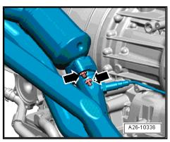
Unscrew nuts in the sequence -9  $\dots$  1- and remove front left exhaust manifold with catalytic converter.
