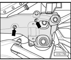
Remove bottom engine/gearbox securing bolts -arrows-.
