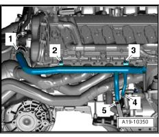
Unscrew bolt -arrow- at bracket for exhaust pipes (right-side).
