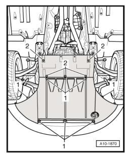
Unscrew bolts -2- on retaining clamps (left and right) for antiroll bar and move anti-roll bar -1- downwards.
