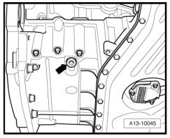
Screw locking pin - 3242- into bore or groove in crankshaft (tightening torque: 20 Nm); if necessary, turn crankshaft backwards and forwards slightly to fully centralise locking pin.
