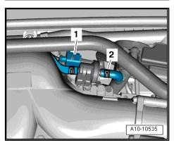
Detach coolant hose -arrow- leading from coolant pipe to coolant expansion tank.
