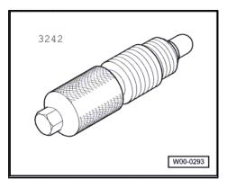
Impact extractor attachment -T10133/3- from tool set for FSI engines - T10133-
