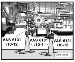
Position support elements from -VAS 6131/10- at right of engine/gearbox assembly, as shown in illustration.
