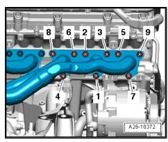
Unscrew nuts in the sequence -6 ... 1- and remove rear right exhaust manifold with catalytic converter.
