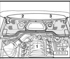
Unbolt bracket (left-side) for refrigerant line from suspension turret -arrow-.
