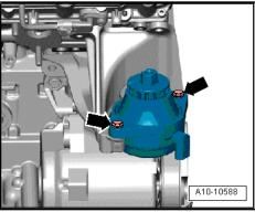
Unscrew bolts -1 ... 5- and remove bracket for torque reaction support.
