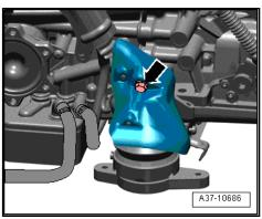
Touch gearbox housing with your hand (without wearing gloves) to eliminate static charge.
