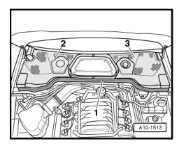
Use screwdriver to pry off caps on wiper arms and slacken off nuts -arrows- several turns.
