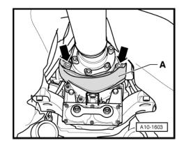
Tie propshaft up to side of heat shield -arrow-.
