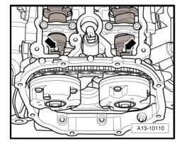
Fit camshaft clamp - T40070- to inlet camshaft and exhaust camshaft as shown in illustration and tighten bolts to 25 Nm.
