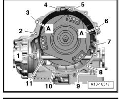
Loosen clamping bolts -1- on sides of scissor-type assembly platform - VAS 6131 A- and pull rear section of platform together with gearbox towards the rear -arrow-; simultaneously separate the torque converter from the drive plate through the opening.
