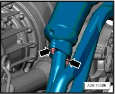
Unscrew nuts in the sequence -9  $\dots$  1- and remove front right exhaust manifold with catalytic converter.
