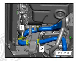
Unscrew nut -1- and remove coolant hose -2- from auxiliary radiator (right-side).
