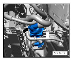
Remove drain plug -arrow- at front coolant pipe and drain off coolant.
