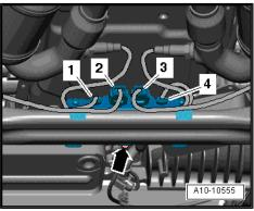
Pull the guide tube for oil dipstick out upwards -arrow-.
