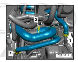
Disconnect coolant hose next to drive shaft (left-side) Projected by copyr coolant pipe -arrow- and drain off coolant.
