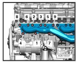
Unplug electrical connector -1- for Lambda probe 4 - G286and move Lambda probe wiring clear.
