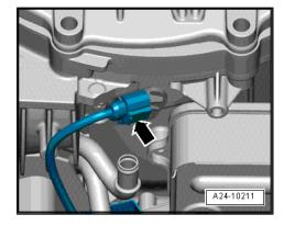
Unbolt bracket for wiring from engine support (right-side) -arrow-.
