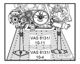
Position support elements from -VAS 6131/10- on engine cross member and subframe (left and right), as shown in illustration.
