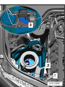
Compress retainer catches -arrows- and detach air duct from lock carrier (front right).
