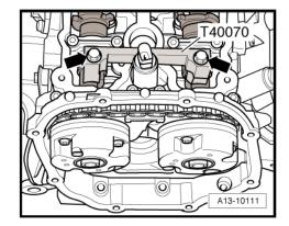
Unscrew plug -arrow- from sump (top section).
