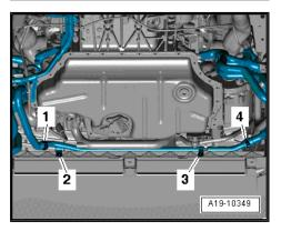
Disconnect hoses -1- and -2- from connecting pipes for secondary air.
