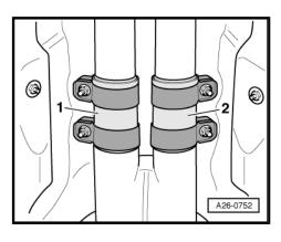
Remove nuts -arrows- and detach front silencer (right-side) from Y-pipe.
