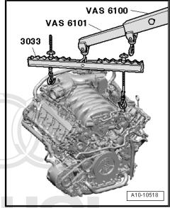
Using bracket -VAS 6095/1-7-, secure engine to engine and gearbox support - VAS 6095- as shown in the illustration. Tightening torque: 42 Nm.
