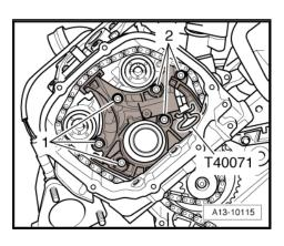
Unscrew bolts -1- and -2- and remove chain tensioner (rightside) and camshaft timing chain (right-side).
