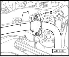
Remove bolts -1, 2, 3- on left and right and detach engine cross member.
