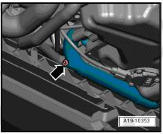
Attach coolant hose (bottom) -2- at auxiliary radiator (righted by copyr side) -arrow-. with respect to the
