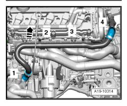
Unscrew bolt -arrow- at bracket for exhaust pipes (left-side).
