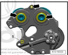
Up to engine number BSM 006 225: Insert spring -2- for drive shaft -3- in spur gear drive -1-.
