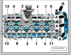
Tighten screw plug -arrow-.
