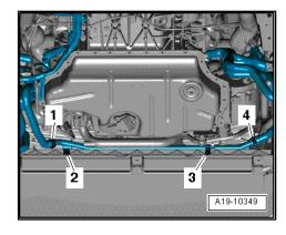
Unscrew bolts -2- and -3- and detach coolant pipe (bottom front) from coolant hoses -1- and -4-.
