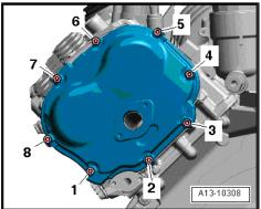
Remove bolts -1 ... 8- and carefully release timing chain cover (right-side) from bonded joint.
