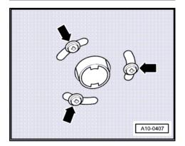
Release quick-release fasteners -1- and -2- and take off noise insulation panels.
