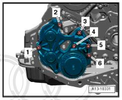
Up to engine number BSM 006 225: Remove spring -2- between spur gear drive -1- and drive shaft -3- for oil pump.
