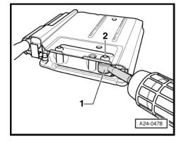
Then grasp head of bolt -2- with vice-grip pliers -1- and unscrew shear bolt in direction of arrow.
