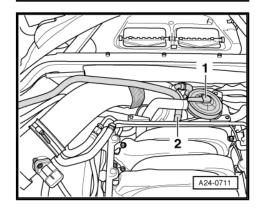
Unscrew bracket from secondary air inlet valve.
