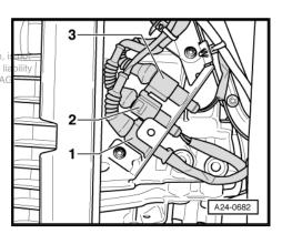
Unscrew Lambda probe using tool from Lambda probe open ring spanner set -3337- .
