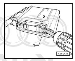
Then grasp head of bolt -2- with vice-grip pliers -1- and unscrew shear bolt in direction of arrow.
