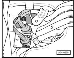
Unscrew the corresponding Lambda probe using tool from Lambda probe open ring spanner set -3337- (illustration shows Lambda probe 2 -G108- on bank 2).
