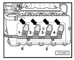
Pull ignition coil (cylinder 1) out with puller -T40039-.
