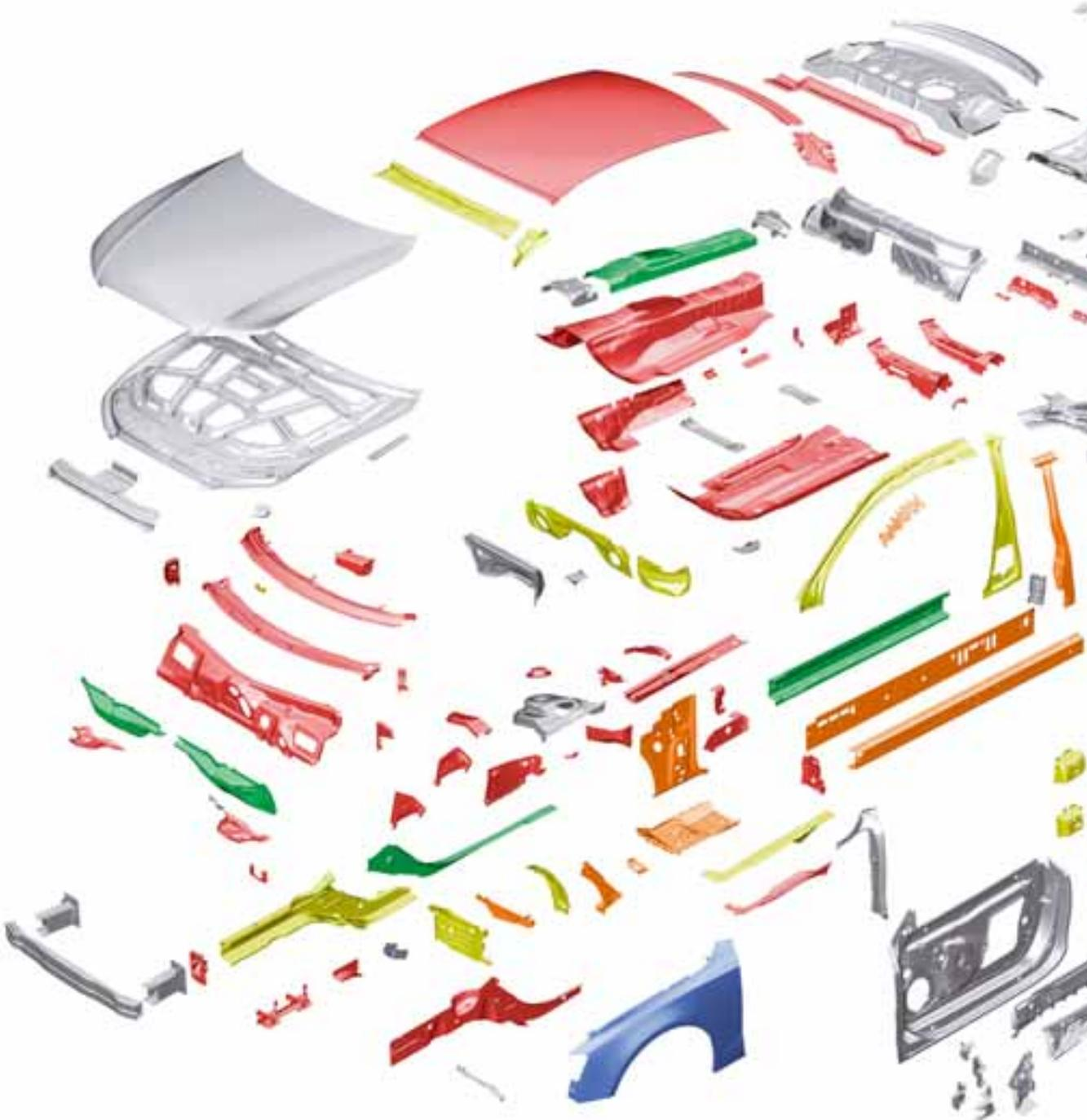
The body construction is a testimony to Audi's experience in lightweight design and its knowledge of innovative welding and joining techniques. Here are examples:
