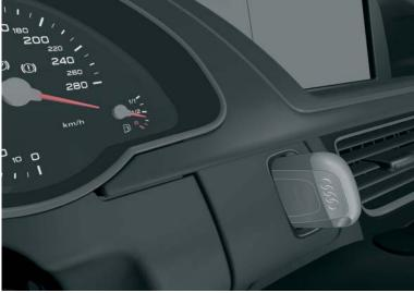
Key inserted in electronic ignition lock module
