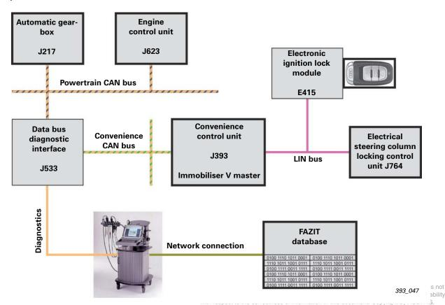
The master for the immobiliser is the convenience system control unit J393, into which the functions of the entry and start authorisation control unit J518 have been integrated. Components which thick borders are all immobiliser system users. Components with thin borders, such as a data bus diagnostic interface and the electronic ignition lock, only transfer immobiliser information.
