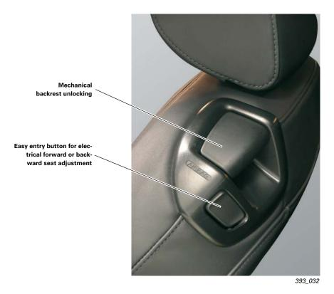
The "easy entry" function allows the front seats to be moved into a position in which the rear seats are more easily accessible.
