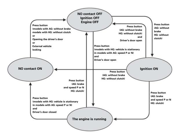
HG ... vehicle with manual gearbox AG ... vehicle with automatic gearbox Button ... Start-Stop button Brake ...Apply the brake Clutch ...Depress the clutch without brake ...do not apply the brake without clutch ...do not depress the clutch
