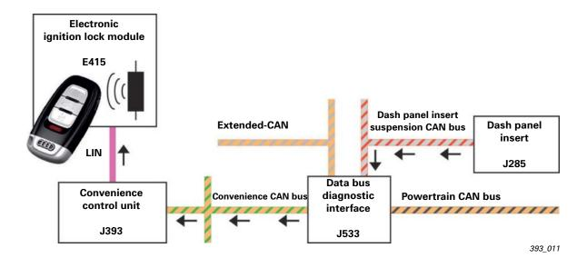
The data for writing to the key is provided by the control unit with display in dash panel insert J285. Data is transferred to the convenience system control unit J393 via the dash panel insert/suspension CAN bus, the data bus diagnostic interface J533 and the convenience CAN bus.
