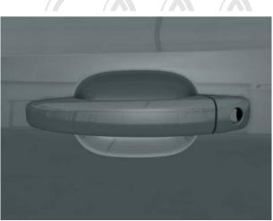
Door outer handle with capacitance sensor
