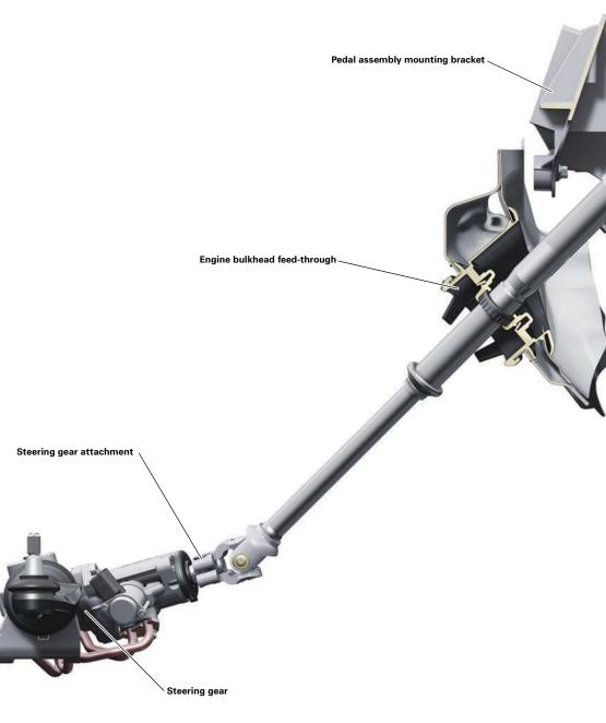
Cutaway view of the steering column as installed
