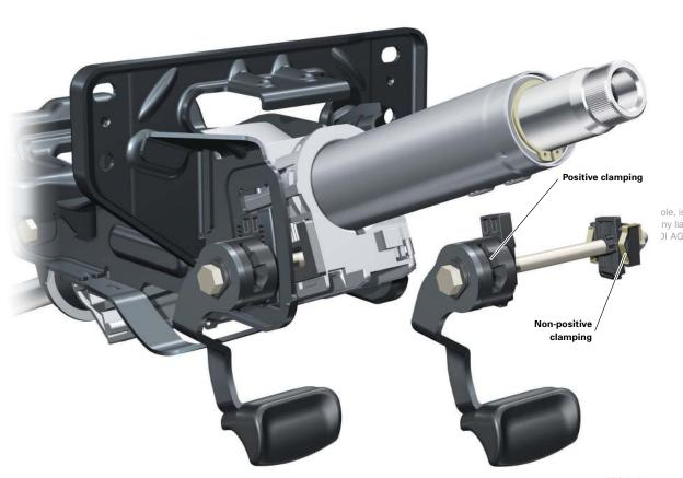
The steering column bracket is connected to the module cross-member at two screw attachment points. The steering column mounting bracket is bolted to the module cross-member, while the steering column bracket is bolted to the mounting bracket. As a result, the steering column attachment points are relatively far apart, creating a broad base which has a positive effect on the vibrational characteristics of the steering column.
