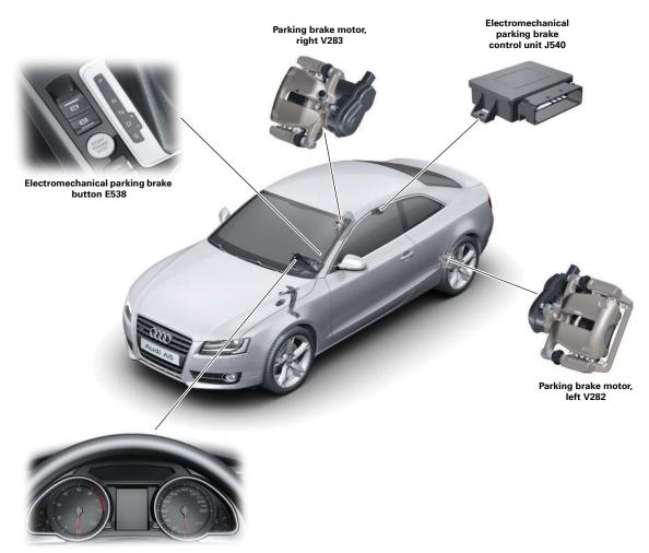
Control unit with display in dash panel insert J285
