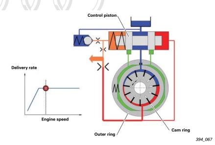
If engine speed continues to increase, both the delivery rate and pressure increase. The control piston displaced further to the left is against the pressure of the spring. As a result, the channel leading to the left chamber is connected to the suction line. The pump pressure flows into the right chamber on the opposite side.
