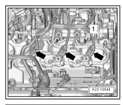
Disconnect fuel return hoses from injectors; to do so, press down both tabs and at the same time pull centre piece up to release connection -arrow-.
