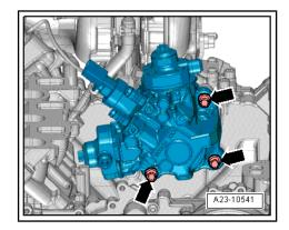
When renewing high-pressure pump, install adapter from old high-pressure pump on new pump. Use counterhold tool -T40248- or counterhold tool -T40292- to loosen and tighten nut -arrow-.
