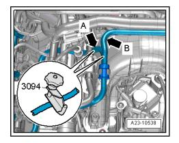
Disconnect fuel return hoses from injectors; to do so, press down both tabs -1 and 2- and at the same time pull centre piece up to release connection -arrow-.
