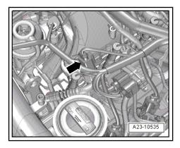
Remove bolts -1 ... 4- and -arrows- and detach intake manifold.
