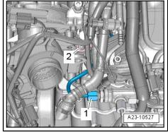
Unplug electrical connector -arrow- at coolant temperature sender -G62-.
