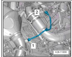
Exhaust gas temperature sender 4 -G648- -arrow- (engine codes CMHA, CPNA only)
