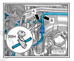
Disconnect fuel return hoses from injectors; to do so, press down both tabs -1 and 2- and at the same time pull centre piece up to release connection -arrow-. Protected by copyright. Copying for private or commercial purposes, in p
