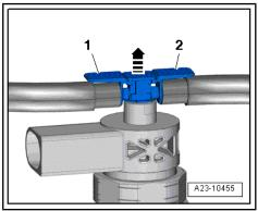
To prevent fuel from being injected when starter is operated, unplug electrical connector at fuel pressure regulating valve -N276- -arrow-.
