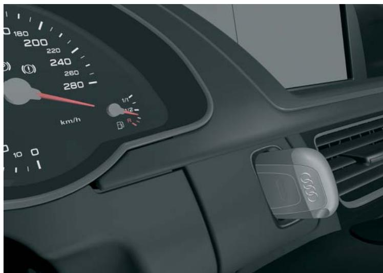
Key inserted in electronic ignition lock module
