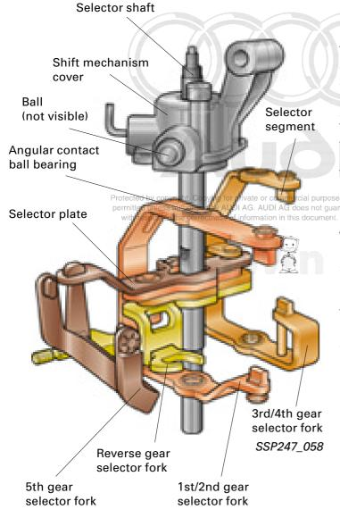
The bearings for the selector forks for 1st/2nd gear and
