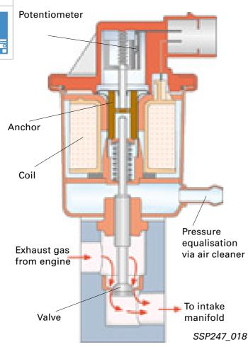
The EGR valve terminates (zero-current process) the recirculation of exhaust gases to the intake manifold. It is switched on from a coolant temperature of 35 °C. When it is actuated, the valve is opened with a defined duty cycle.
