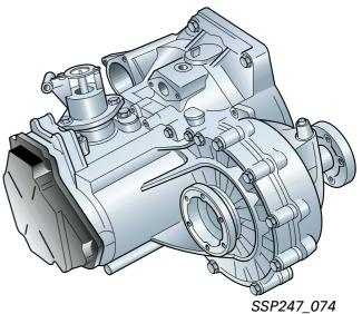
The familiar 02J gearbox is used in the A2 1.4 I TDI, for torques up to 250 Nm.
