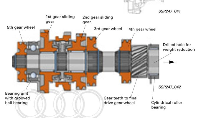
The gear wheels for the 3rd, 4th and 5th gears and the 1st/2nd gear synchro-hub are attached via fine teeth. The sliding gears of the 1st and 2nd gears run on needle roller bearings on the output shaft.
