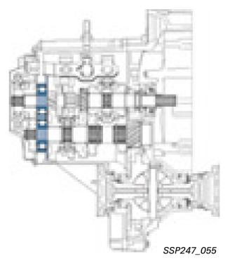
The complete package of shafts and gear wheels for the input shaft and the output shaft is pre-assembled outside the gearbox housing in the bearing support, and can then be easily inserted into the gearbox housing.
