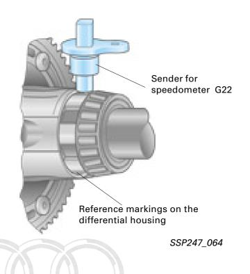
The sender operates in accordance with the Hall sender principle. The PWM signal (pulse width modulated) is sent to the combiprocessor in dash panel insert J218.
