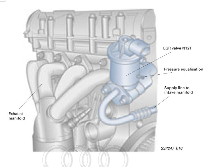
EGR valve N121 is electrically controlled and actuated directly by engine control unit J537.
