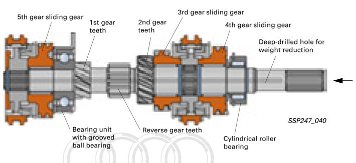
The teeth for 1st gear, 2nd gear and reverse gear are permanently connected to the input shaft. The synchro-hubs for the 3rd/4th gear and the 5th gear are attached via fine teeth.
