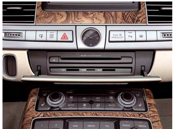
Control unit for information electronics 1 J794 in the centre console
