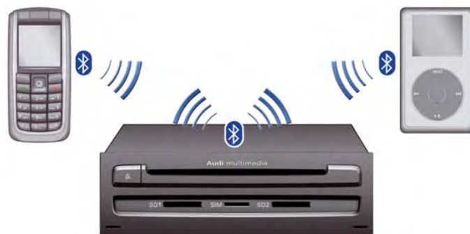
Parallel connection of two terminal devices with J794 via Bluetooth
