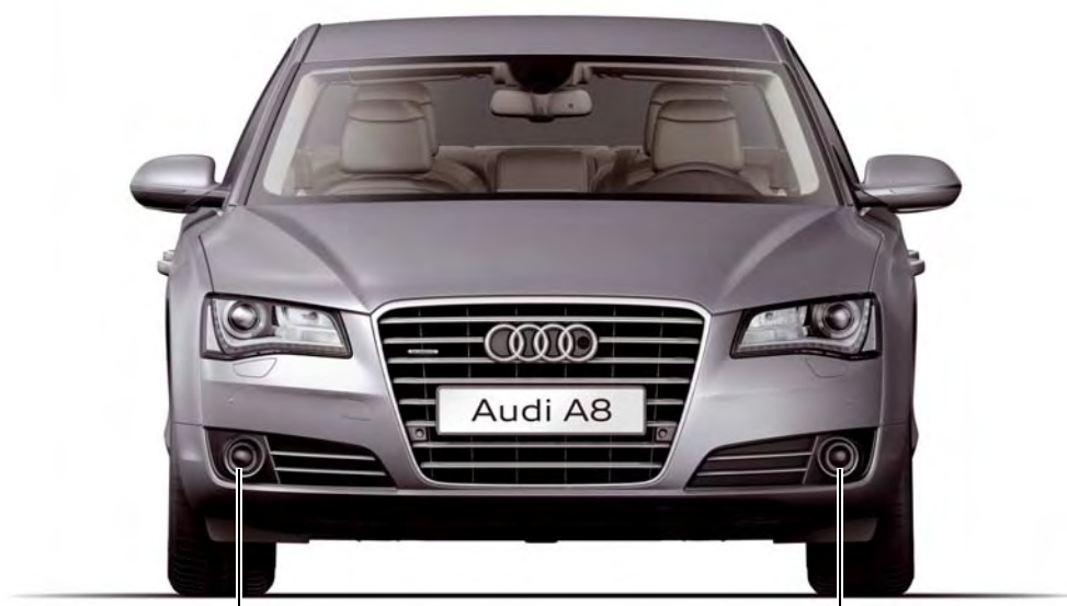
ADC sender, right G259 and ACC control unit J428
