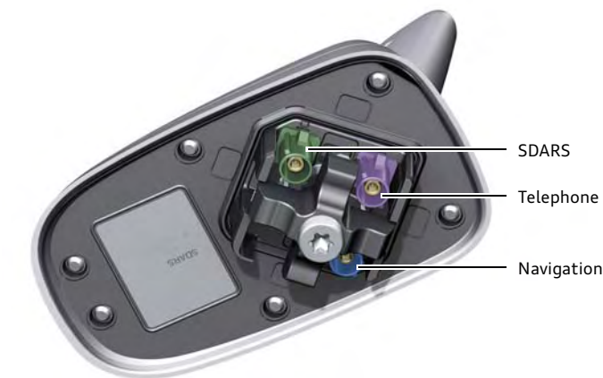
Roof antenna R216 (North America)
